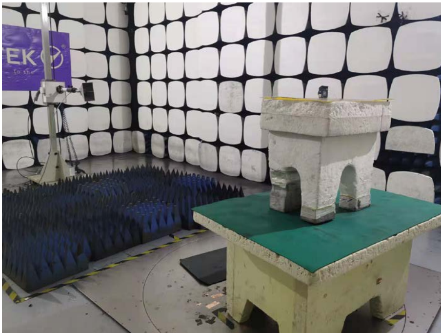
Spurious Emission Test Setup (Above 1GHz)
