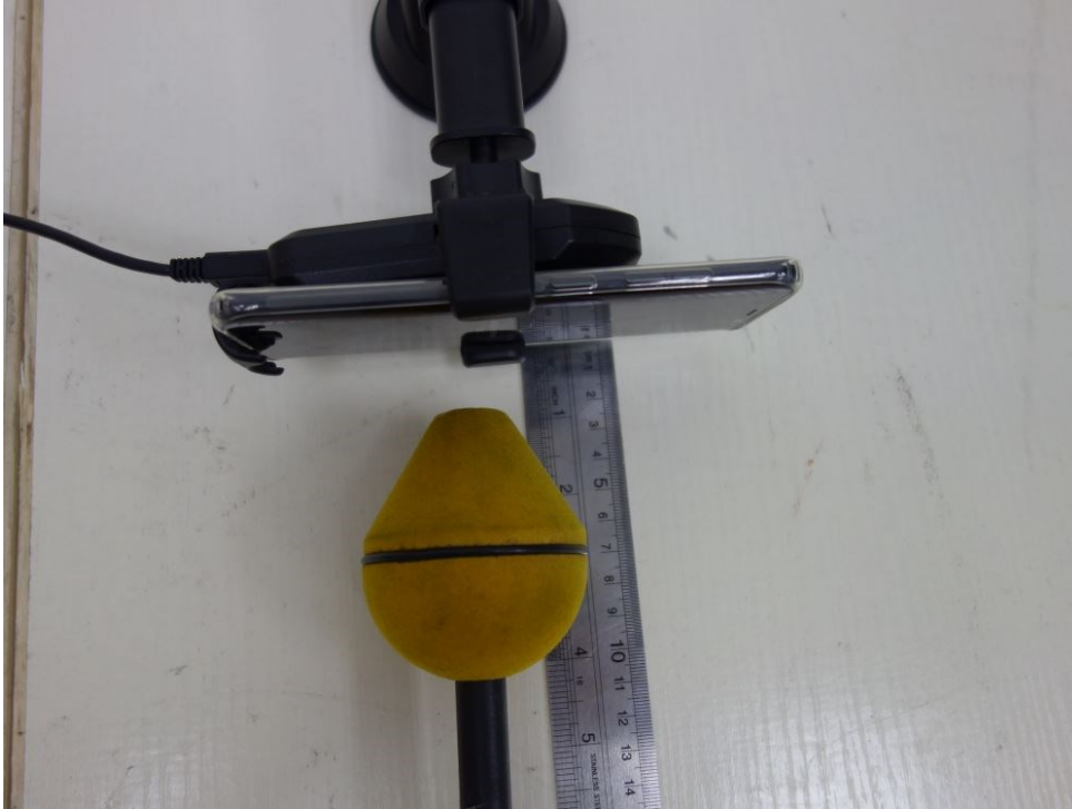
Side Top test distance at 9cm
