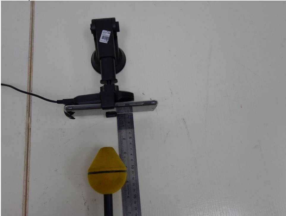
Side Top test distance at 13cm
