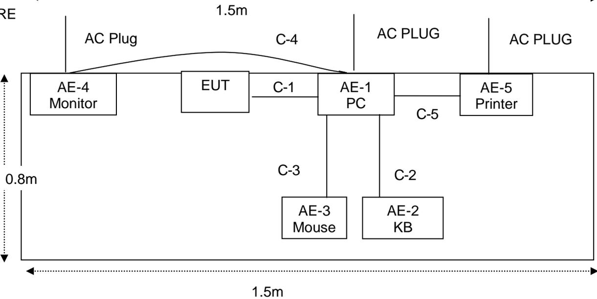
**2.3 DESCRIPTION TEST PERIPHERAL AND EUT PERIPHERAL**
