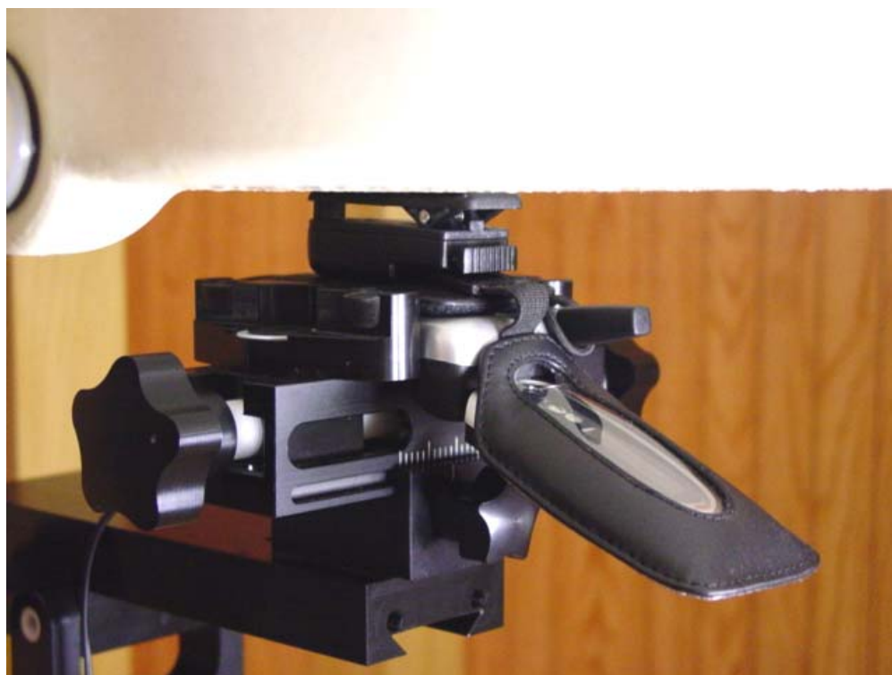
Figure 12.7 body SAR setup open (with leather case)
