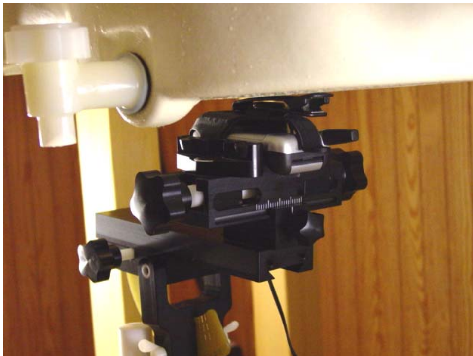
Figure 12.3 body SAR setup closed (with holster)
