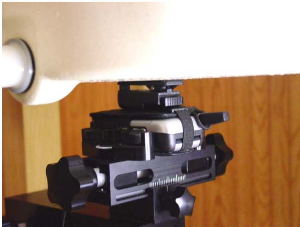
Figure 12.7 body SAR setup closed (with leather case)
