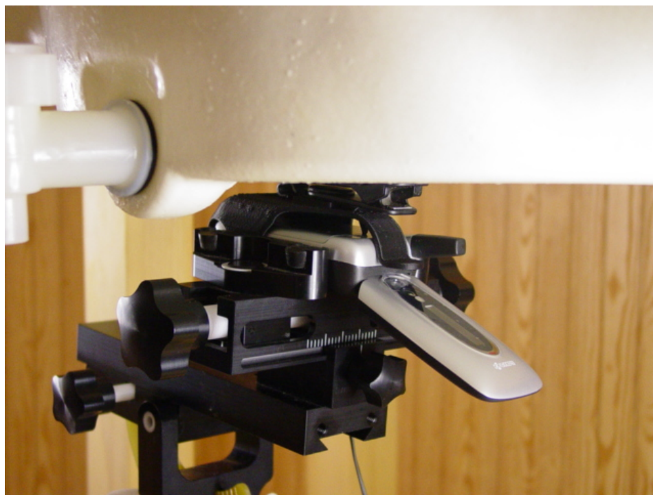
Figure 12.4 body SAR setup open (with holster)
