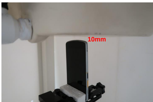
Bottom Side, Test Separation 10 mm
