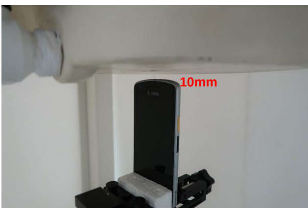
Top Side, Test Separation 10 mm
