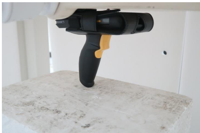
Front with Soft Holster + Trigger Handle, Test Separation 0 mm
