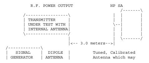
Equipment placed 1 meter above ground on a rotatable platform
