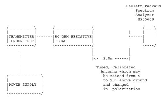
Equipment placed 4' above ground on a rotatable platform.
