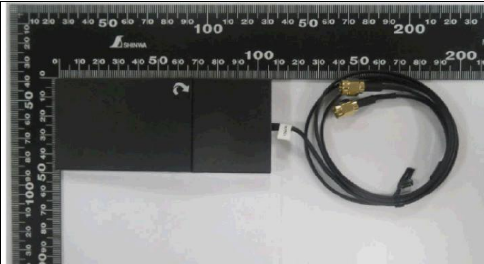
Antenna set 2 (Brand : INPAQ, Model : DAM-I6-H-DB-800-10-17)
