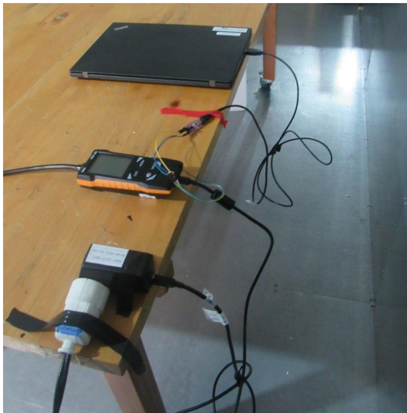
Powerline test setup
