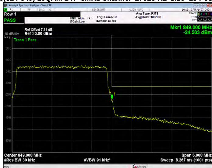
Band26(824-849) 16QAM BW=5MHz Channel=26815 RB Size=25 Position=#0
