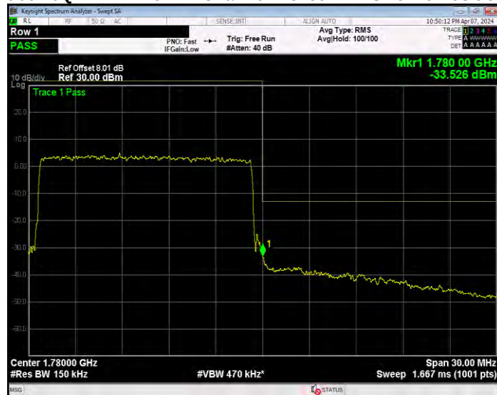
Band66 16QAM BW=20MHz Channel=132072 RB Size=1 Position=#0
