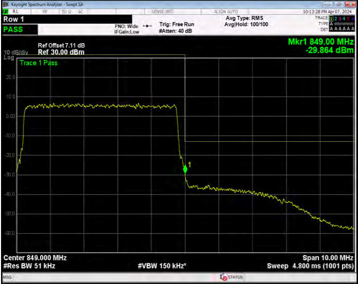
Band66 16QAM BW=1.4MHz Channel=131979 RB Size=1 Position=#0
