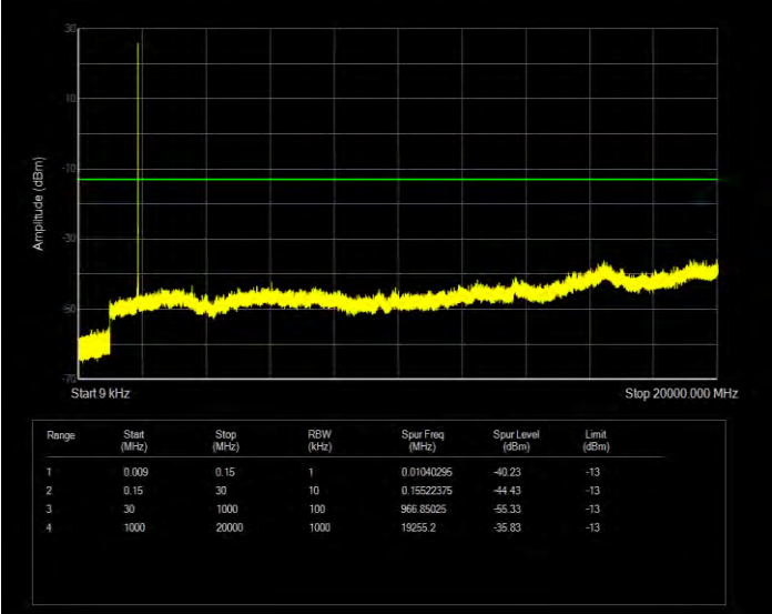
Band2 16QAM BW=1.4MHz Channel=19193 RB Size=6 Position=#0
