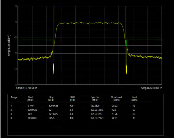
Band26(814-824) QPSK BW=5MHz Channel=26715 RB Size=25 Position=#0
