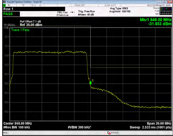
Band26(824-849) 16QAM BW=15MHz Channel=26865 RB Size=75 Position=#0
