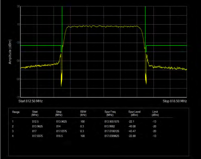
Band26(814-824) 16QAM BW=3MHz Channel=26775 RB Size=15 Position=#0
