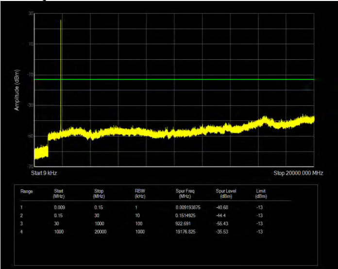
Band2 16QAM BW=1.4MHz Channel=19193 RB Size=6 Position=#0
