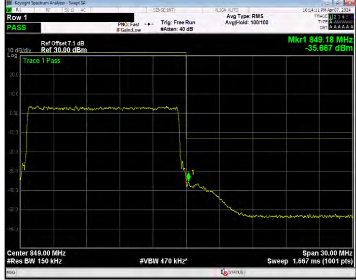
Band26(824-849) 16QAM BW=15MHz Channel=26965 RB Size=75 Position=#0
