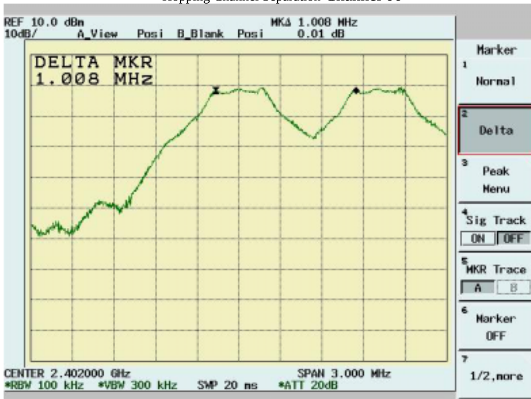
Hopping Channel Separation Channel 00
