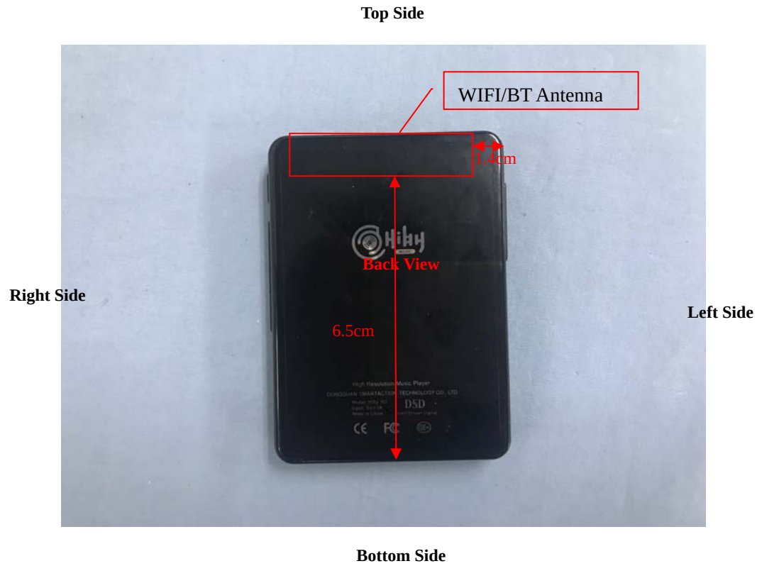
Fig 7.1 Block Diagram for EUT Antenna Position
