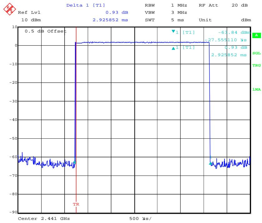
*EDR Mode (8DPSK):***3DH1: Middle Channel**
