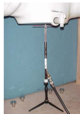
835 MHz Dipole Setup
