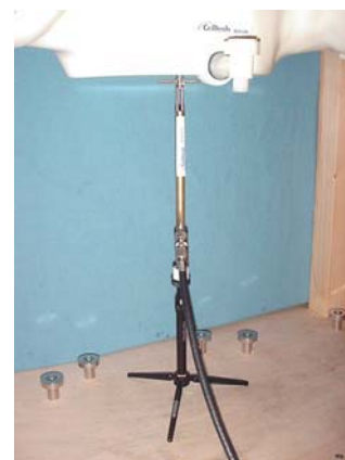
1900 MHz Dipole Setup
