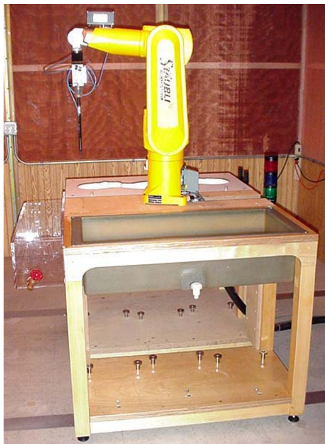
DASY4 SAR Measurement System with Planar Phantom
