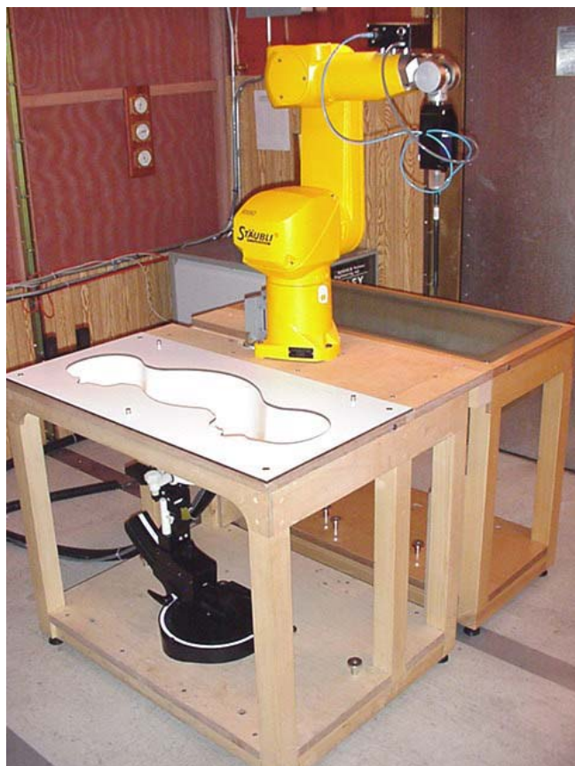
DASY4 SAR Measurement System with SAM Phantom
