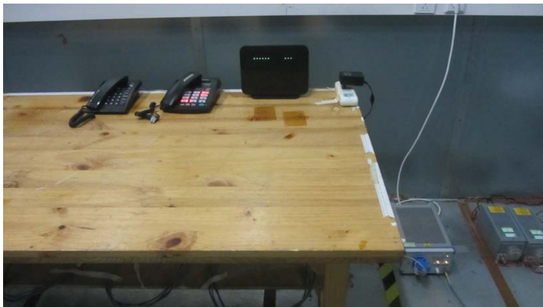
Picture 3 Conducted Emission Test Setup
