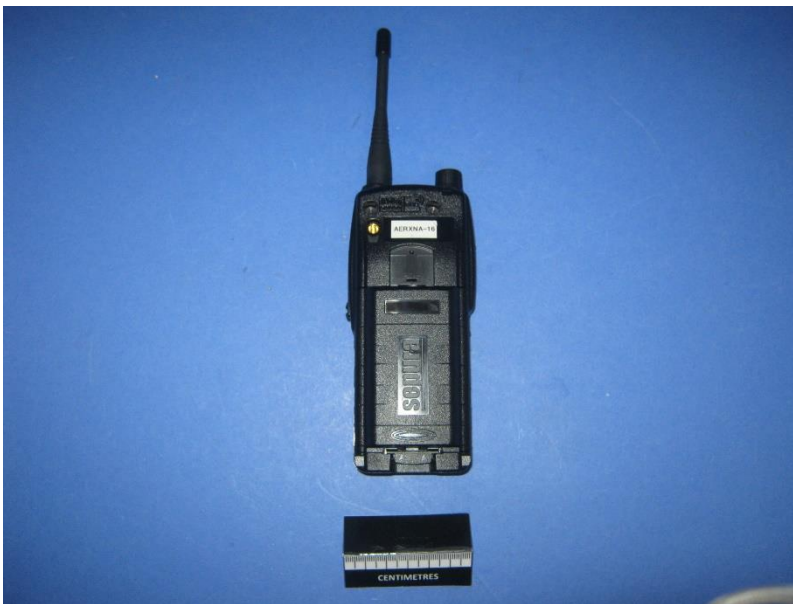
Figure 51 Rear – 1880 mAh battery Fitted
