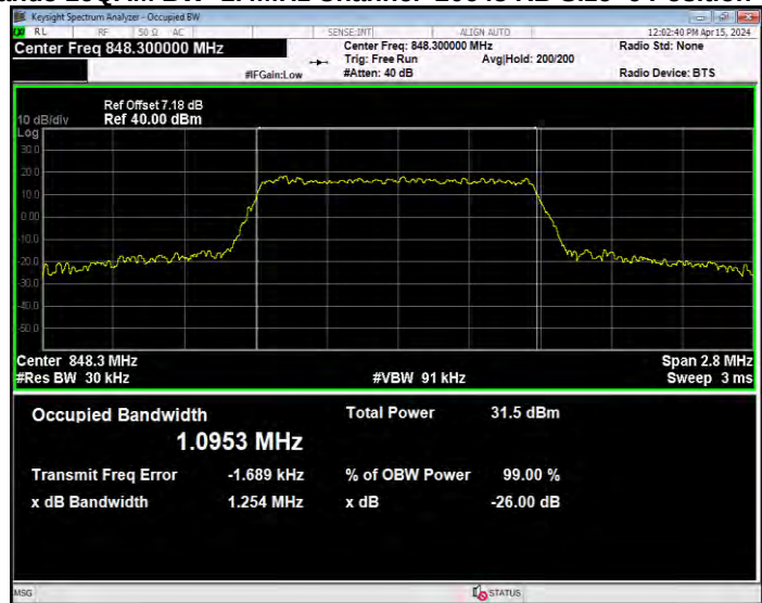
Band5 16QAM BW=10MHz Channel=20450 RB Size=50 Position=#0
