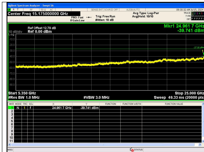
Spurious Emission:5350~25000.0 MHz IEEE 802.11n_Channel 38_40MHz_Antenna 0
