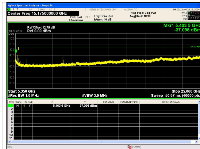
Spurious Emission:5350~25000.0 MHz IEEE 802.11n_Channel 40_20MHz_Antenna 0
