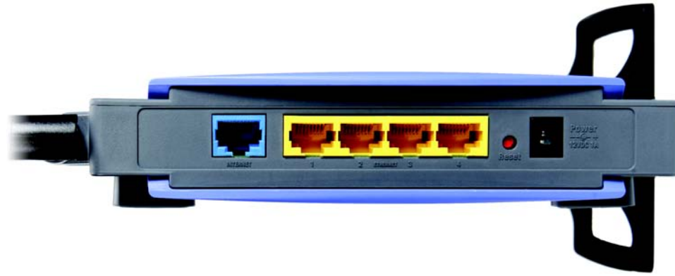
Figure 3-1: The Router's Back Panel
