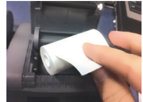
INCORRECT Roll Orientation
