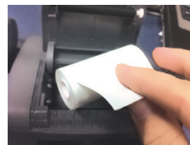
Incorrect roll orientation
