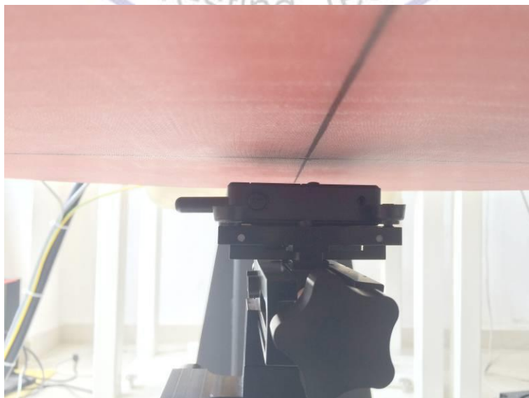
Face-held, the front of the EUT towards phantom (The distance is 25mm)
