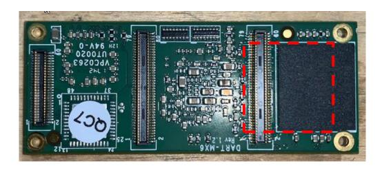
Note: The red outline shows the PQG-XREADER2 device boundaries. It does not include the Variscite DART-MX6 computer module.
