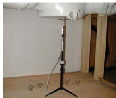
Figure 9.1 Dipole Verification Test Setup Diagram & Photo
