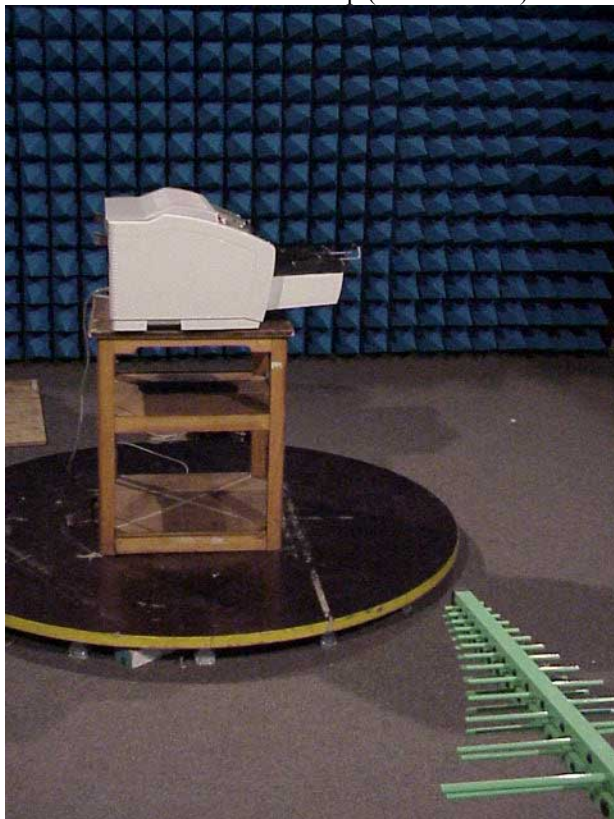
Photo 2: radiated emission set-up (30-1000MHz)
