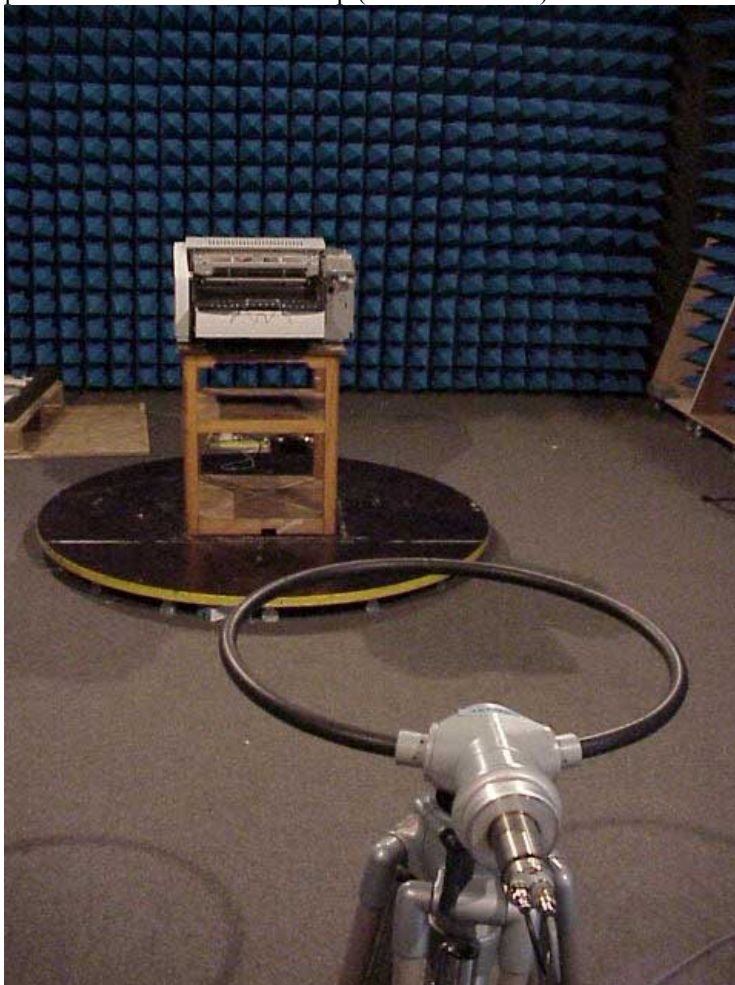
photo 5 radiated emission set-up (band 13.56MHz)
