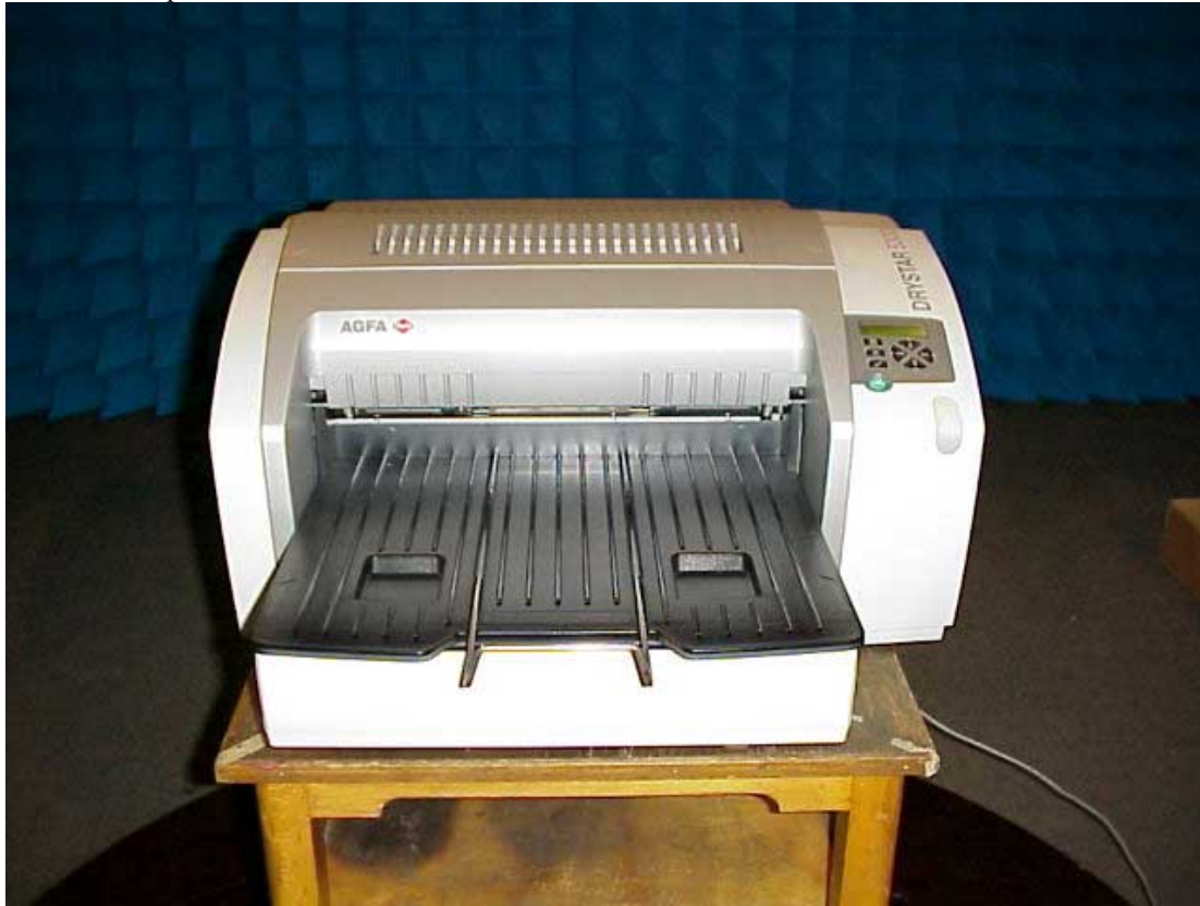
Photo 2: radiated emission set-up (30-1000MHz)
