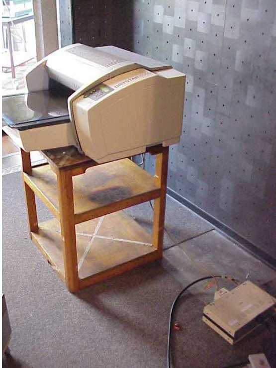
photo 5 radiated emission set-up (band 13.56MHz)
