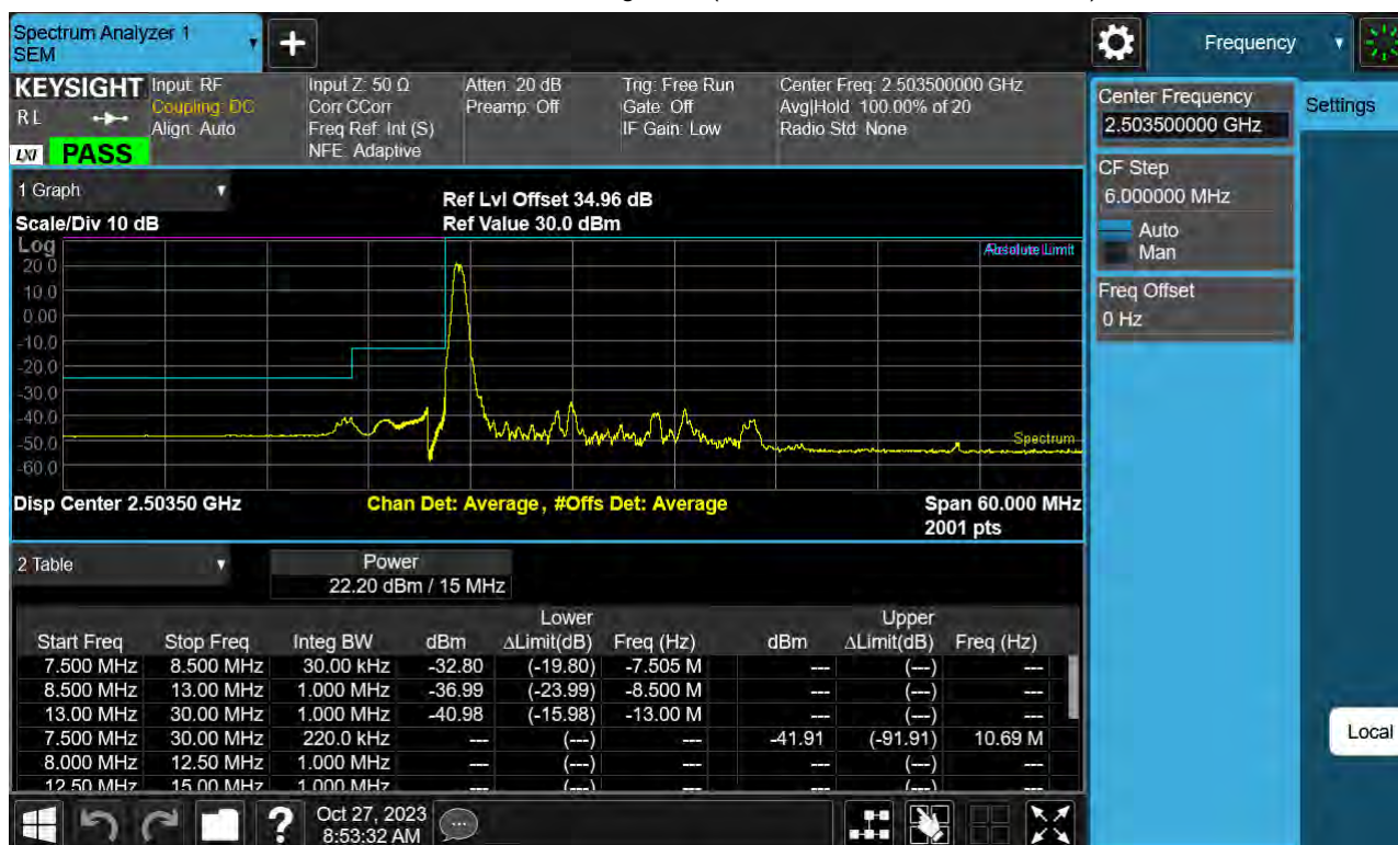
Sub6 n41. Low Channel Edge Plot (15 MHz Ch.500700 BPSK RB 1)-1
