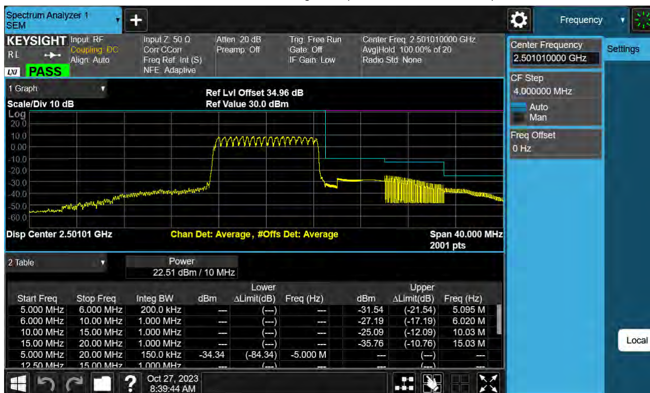
Sub6 n41. Low Channel Edge Plot (10 MHz Ch.500202 BPSK)-2
