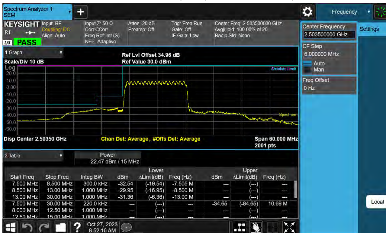
Sub6 n41. Low Channel Edge Plot (15 MHz Ch.500700 BPSK )-1
