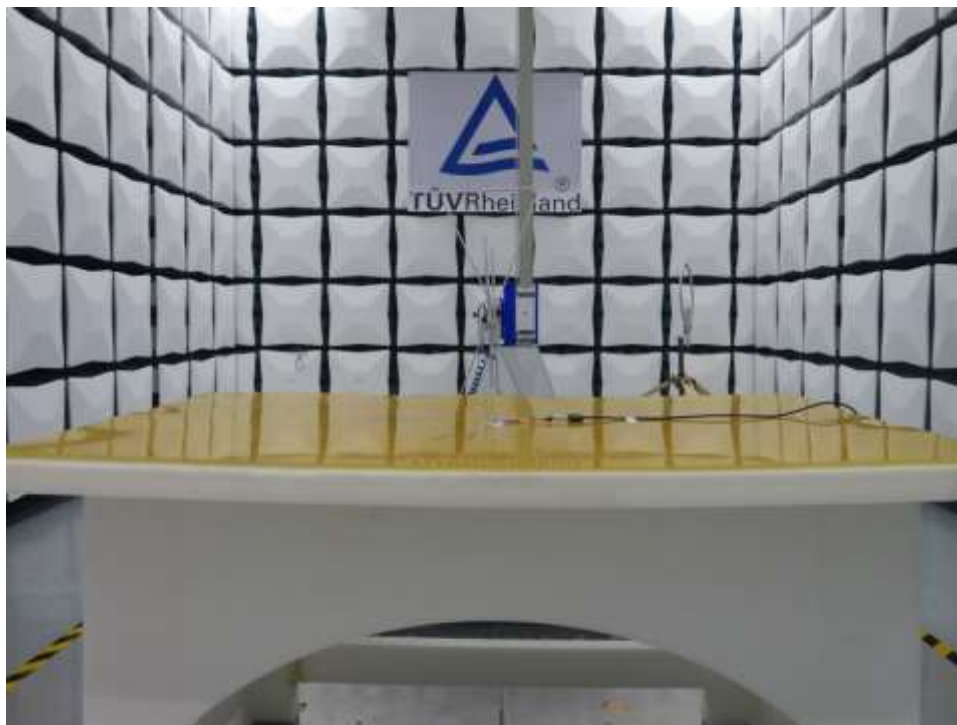
Photograph 1: Set-up photo for Radiated Emissions Below 1GHz
