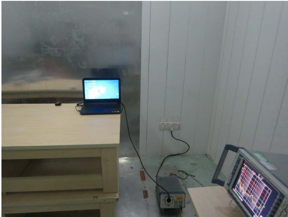
FCC RADIATED EMISSION TEST SETUP
