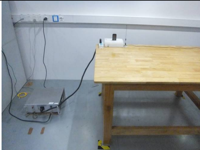
Conducted Emissions Test Setup Front View
