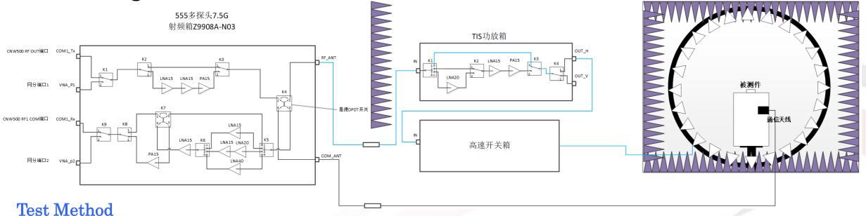
The "great circle" cut method, whereby the Measurement Antenna remains fixed and the EUT is rotated about two axes in sequential order. The radiated RF performance of the Equipment Under Test (EUT) is measured by sampling the radiated transmit power of the mobile at various locations surrounding the device. A three-dimensional characterization of the 'transmit' performance of the EUT is pieced together by analyzing the data from the spatially distributed measurements.
