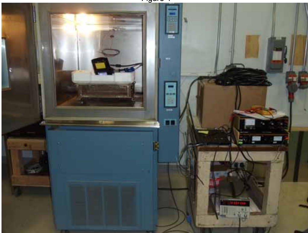
Test Setup for Frequency Stability Tests
