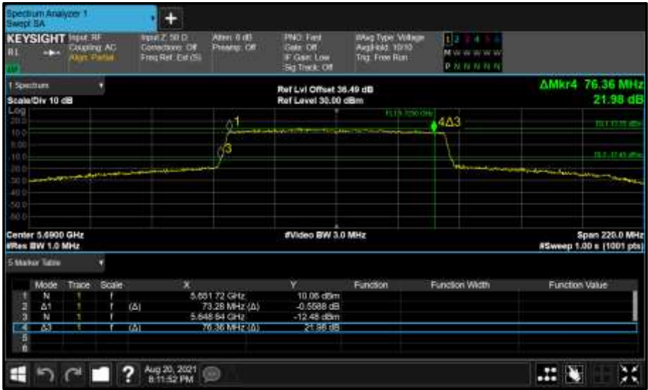
Figure 578 - Core 1 (B) 5690 MHz (CH138) 26 dB and 99% Bandwidth
