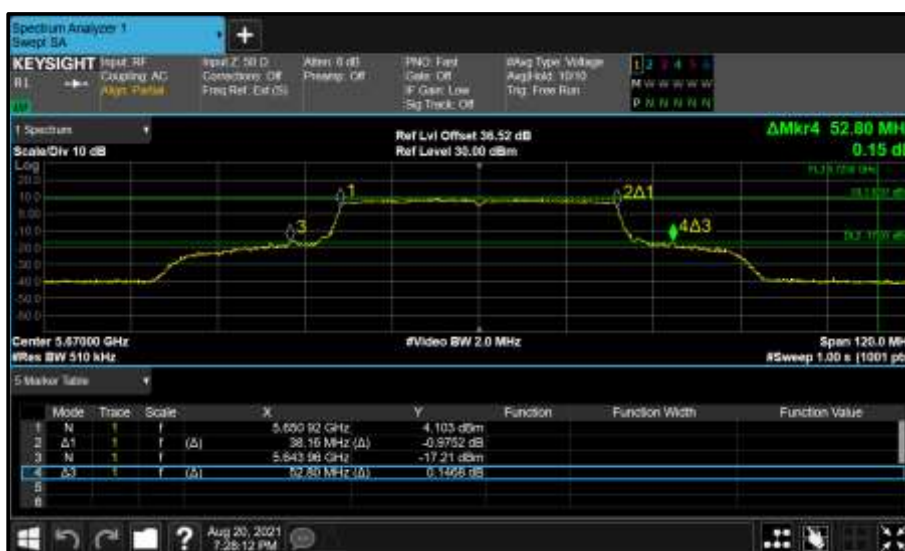
Figure 558 - Core 1 (B) 5670 MHz (CH134) 26 dB and 99% Bandwidth
