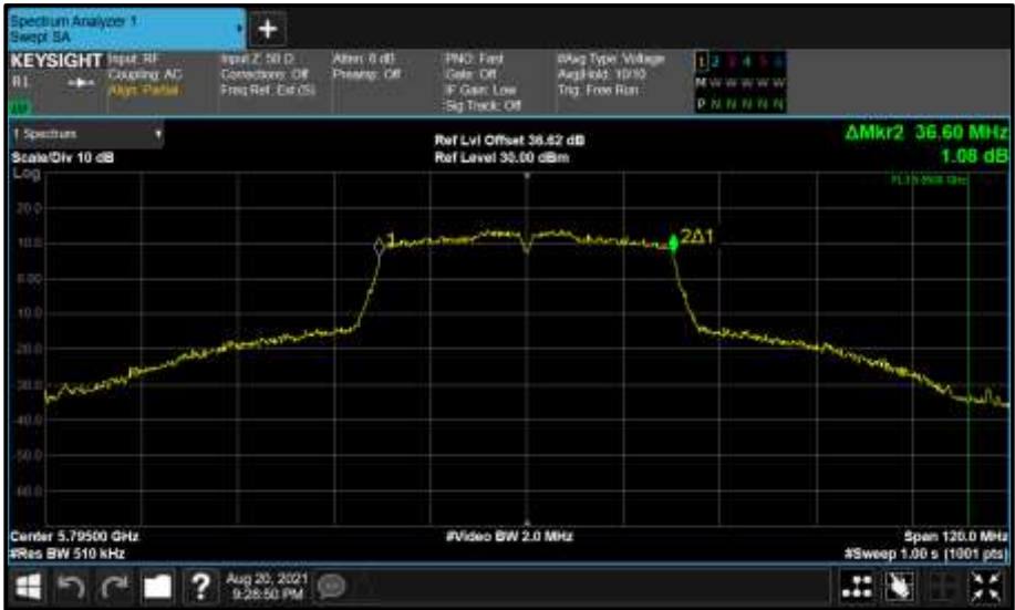
Figure 677 - Core 1 (B) 5795 MHz (CH159) 99% Bandwidth
