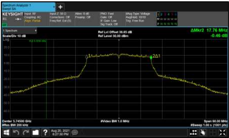
Figure 611 - Core 1 (B) 5745 MHz (CH149) 99% Bandwidth
