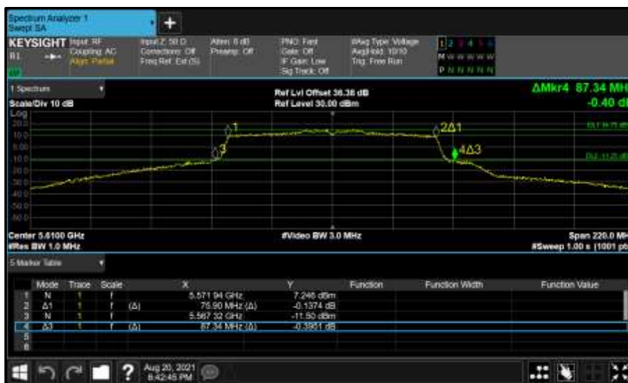
Figure 475 - Core 0 (A) 5610 MHz (CH122) 26 dB and 99% Bandwidth
