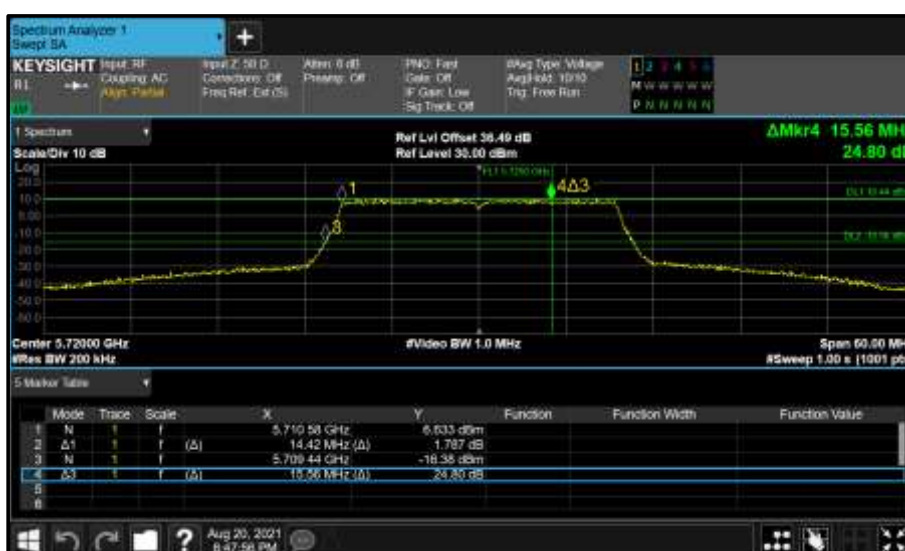
Figure 492 - Core 0 (A) 5720 MHz (CH144) 26 dB and 99% Bandwidth
