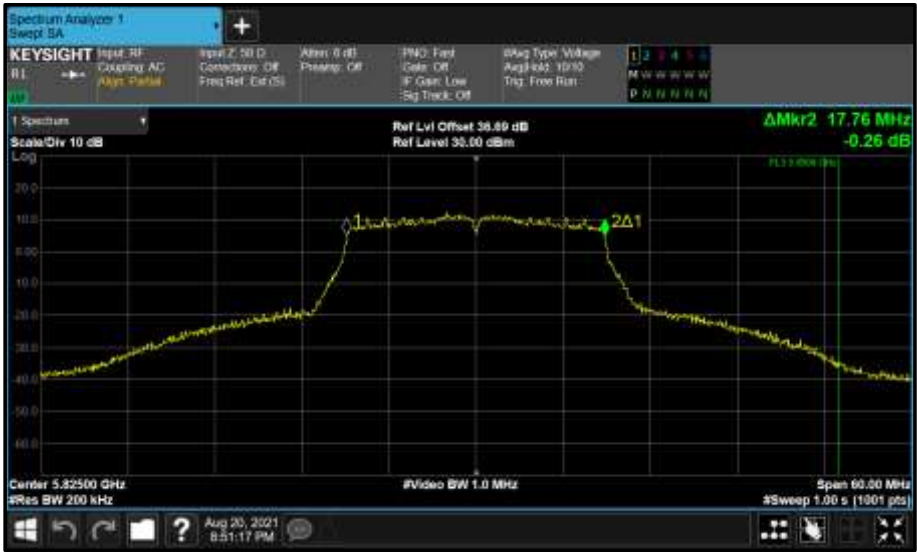
Figure 629 - Core 0 (A) 5825 MHz (CH165) 99% Bandwidth
