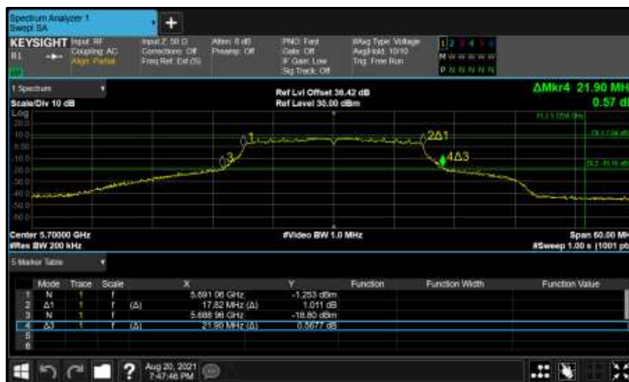
Figure 450 - Core 0 (A) 5700 MHz (CH140) 26 dB and 99% Bandwidth
