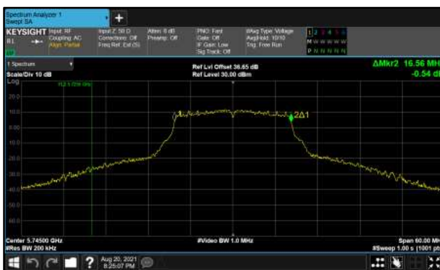
Figure 603 - Core 1 (B) 5745 MHz (CH149) 99% Bandwidth
