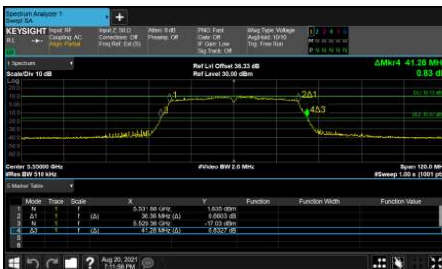
Figure 461 - Core 1 (B) 5550 MHz (CH110) 26 dB and 99% Bandwidth
