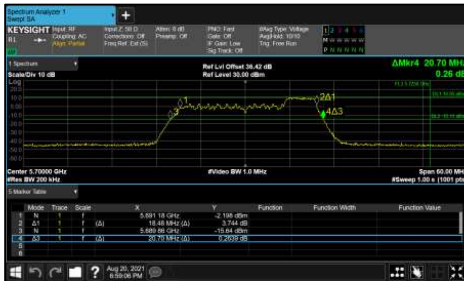
Figure 511 - Core 0 (A) 5700 MHz (CH140) 26 dB and 99% Bandwidth
