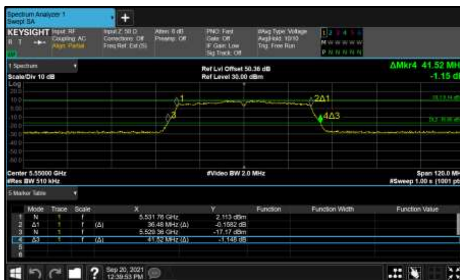
Figure 590 - Core 1 (B) 5550 MHz (CH110) 26 dB and 99% Bandwidth
