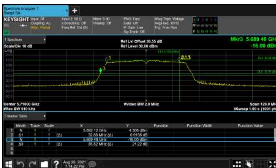
Figure 465 - Core 1 (B) 5710 MHz (CH142) 26 dB and 99% Bandwidth
