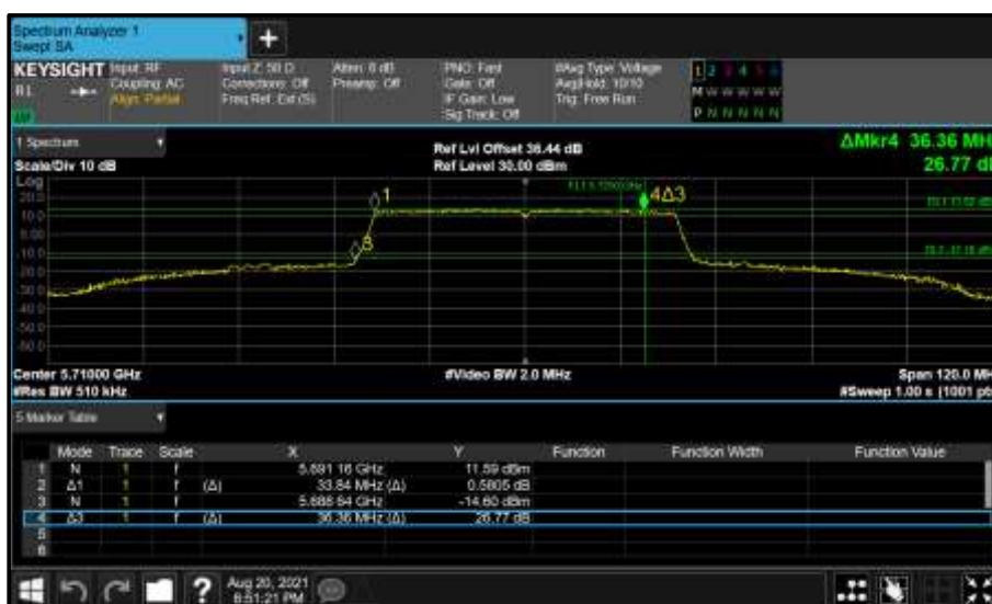
Figure 552 - Core 0 (A) 5710 MHz (CH142) 26 dB and 99% Bandwidth
