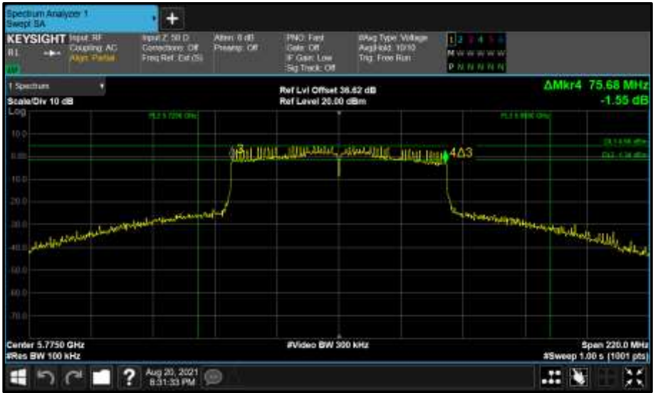
Figure 682 - Core 1 (B) 5775 MHz (CH155) 6 dB Bandwidth
