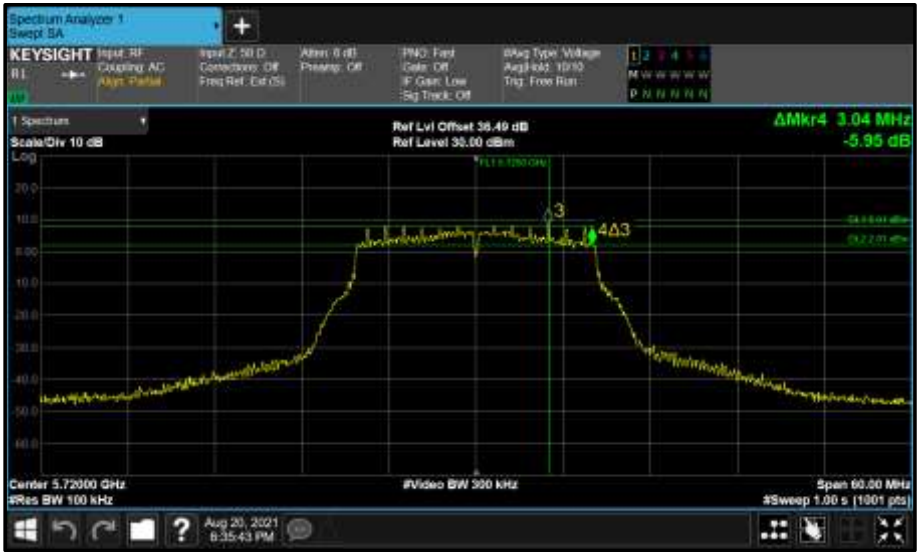
Figure 602 - Core 0 (A) 5720 MHz (CH144) 6 dB Bandwidth
