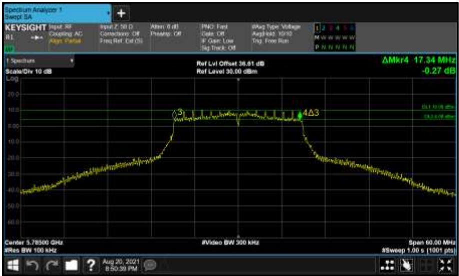
Figure 628 - Core 1 (B) 5785 MHz (CH157) 6 dB Bandwidth
