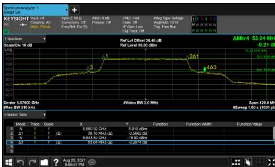
Figure 565 - Core 0 (A) 5670 MHz (CH134) 26 dB and 99% Bandwidth
