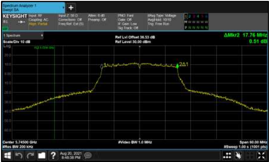
Figure 621 - Core 0 (A) 5745 MHz (CH149) 99% Bandwidth
