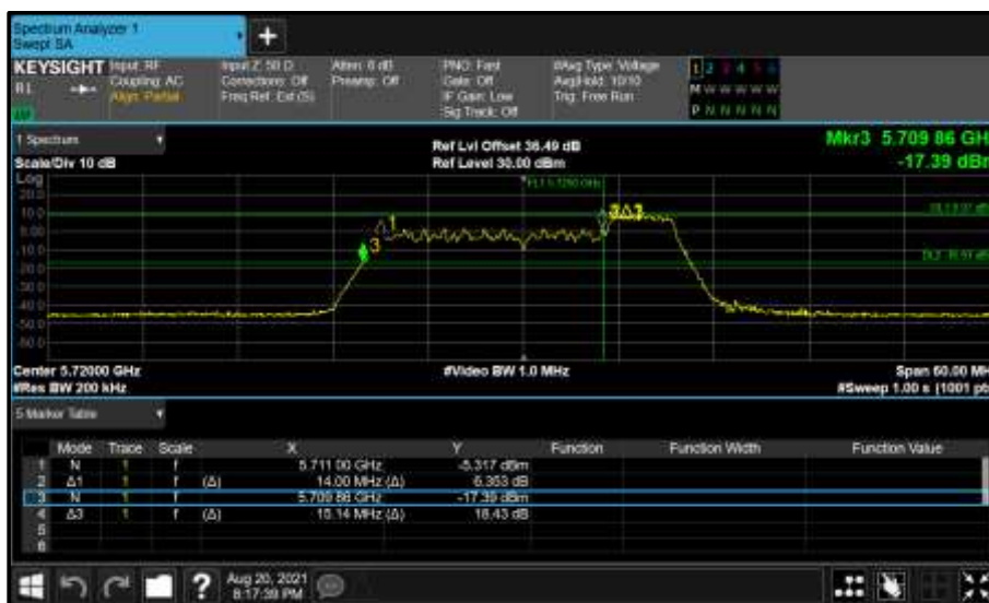
Figure 527 - Core 0 (A) 5720 MHz (CH144) 26 dB and 99% Bandwidth
