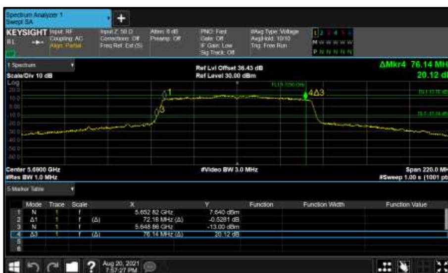
Figure 487 - Core 0 (A) 5690 MHz (CH138) 26 dB and 99% Bandwidth
