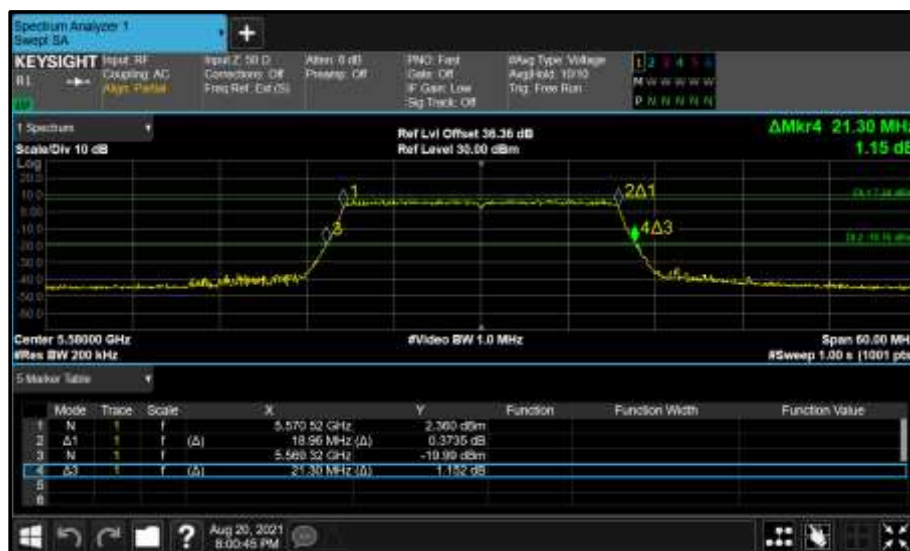
Figure 504 - Core 1 (B) 5580 MHz (CH116) 26 dB and 99% Bandwidth
