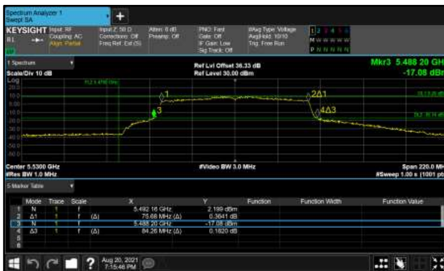
Figure 478 - Core 1 (B) 5530 MHz (CH106) 26 dB and 99% Bandwidth
