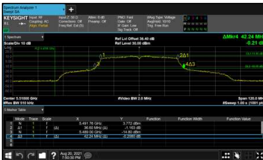
Figure 466 - Core 0 (A) 5510 MHz (CH102) 26 dB and 99% Bandwidth
