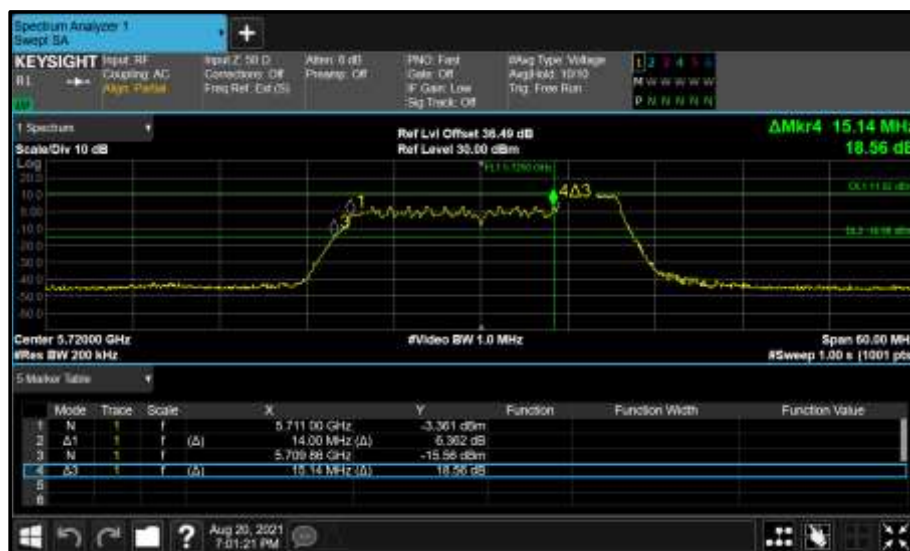
Figure 512 - Core 0 (A) 5720 MHz (CH144) 26 dB and 99% Bandwidth
