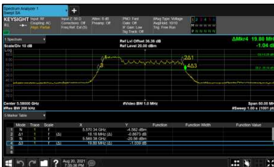
Figure 516 - Core 1 (B) 5580 MHz (CH116) 26 dB and 99% Bandwidth
