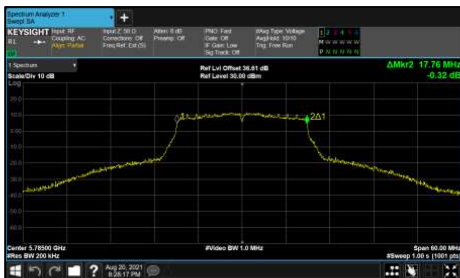
Figure 613 - Core 1 (B) 5785 MHz (CH157) 99% Bandwidth
