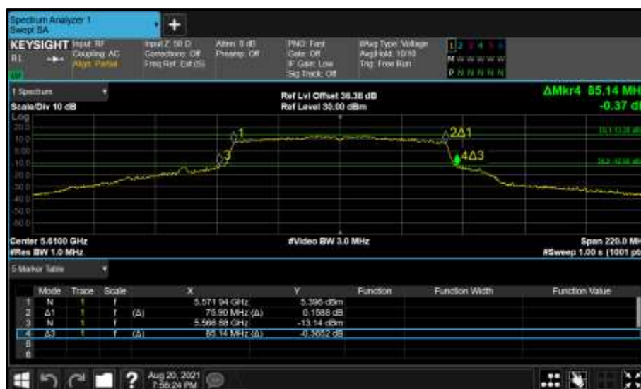
Figure 485 - Core 0 (A) 5610 MHz (CH122) 26 dB and 99% Bandwidth
