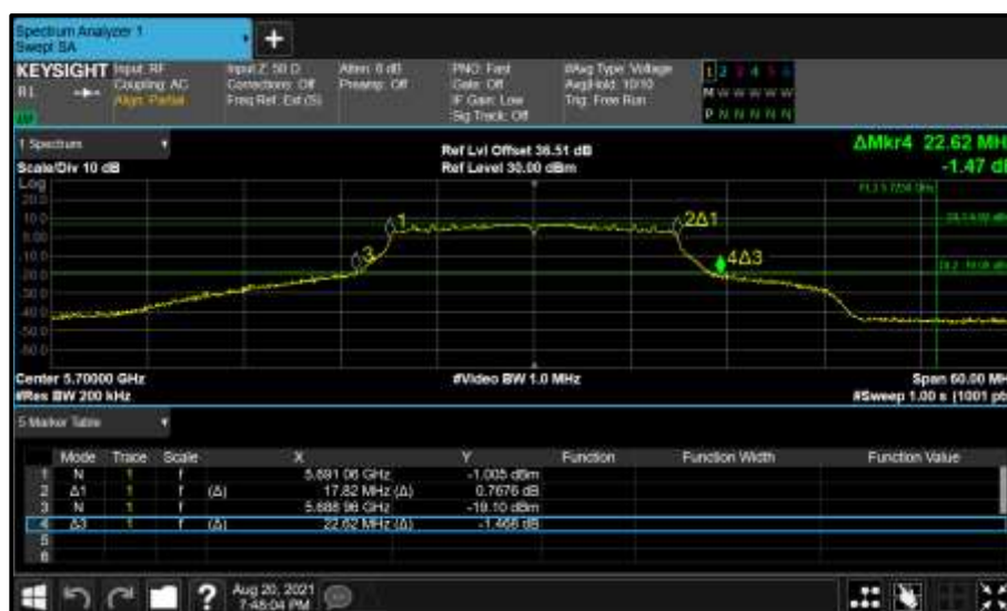
Figure 451 - Core 1 (B) 5700 MHz (CH140) 26 dB and 99% Bandwidth
