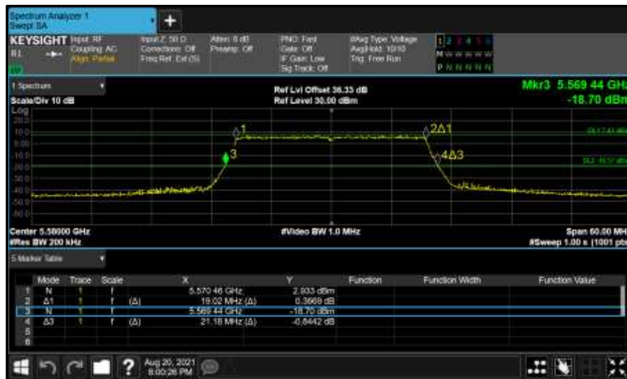
Figure 503 - Core 0 (A) 5580 MHz (CH116) 26 dB and 99% Bandwidth
