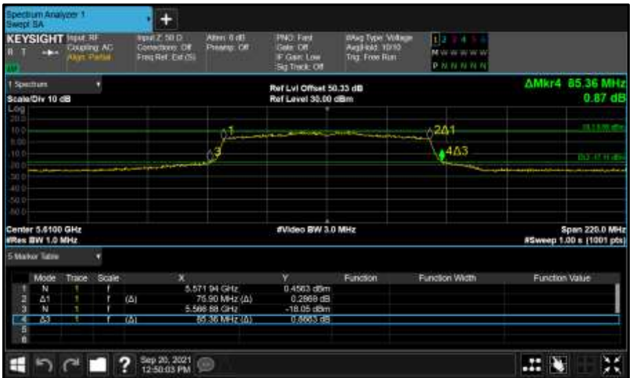
Figure 597 - Core 0 (A) 5610 MHz (CH122) 26 dB and 99% Bandwidth
