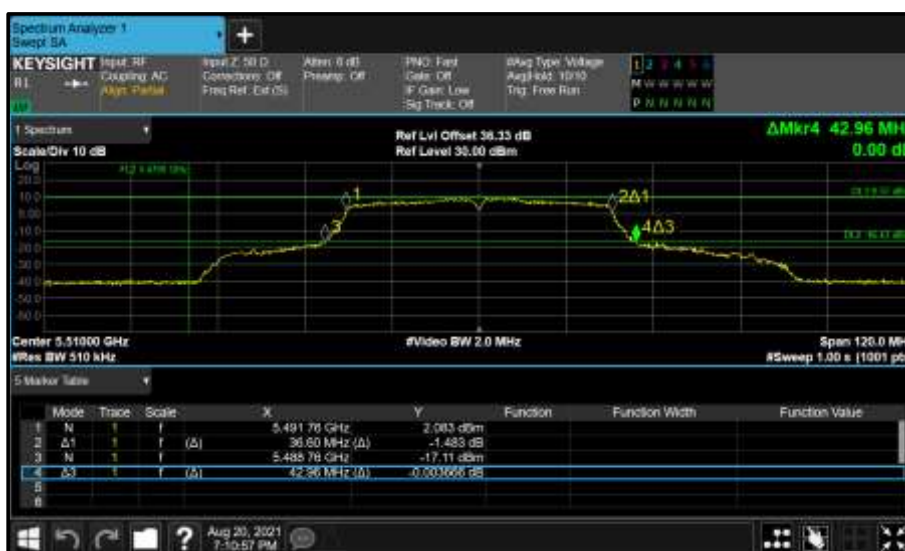
Figure 459 - Core 1 (B) 5510 MHz (CH102) 26 dB and 99% Bandwidth
