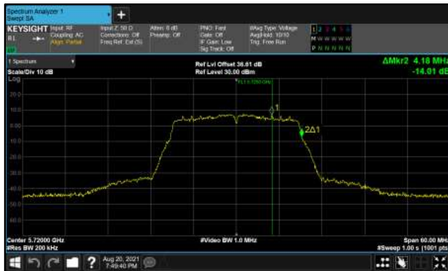
Figure 635 - Core 1 (B) 5720 MHz (CH144) 99% Bandwidth
