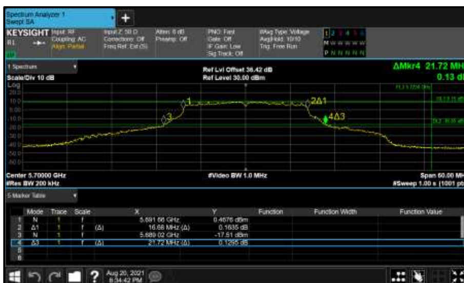
Figure 432 - Core 0 (A) 5700 MHz (CH140) 26 dB and 99% Bandwidth
