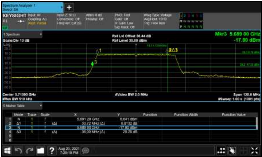
Figure 559 - Core 0 (A) 5710 MHz (CH142) 26 dB and 99% Bandwidth
