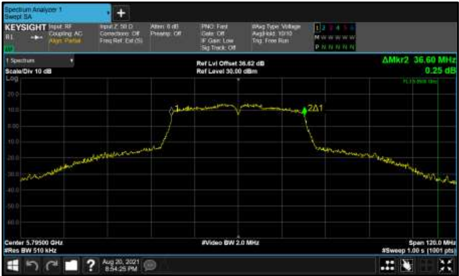
Figure 665 - Core 1 (B) 5795 MHz (CH159) 99% Bandwidth
