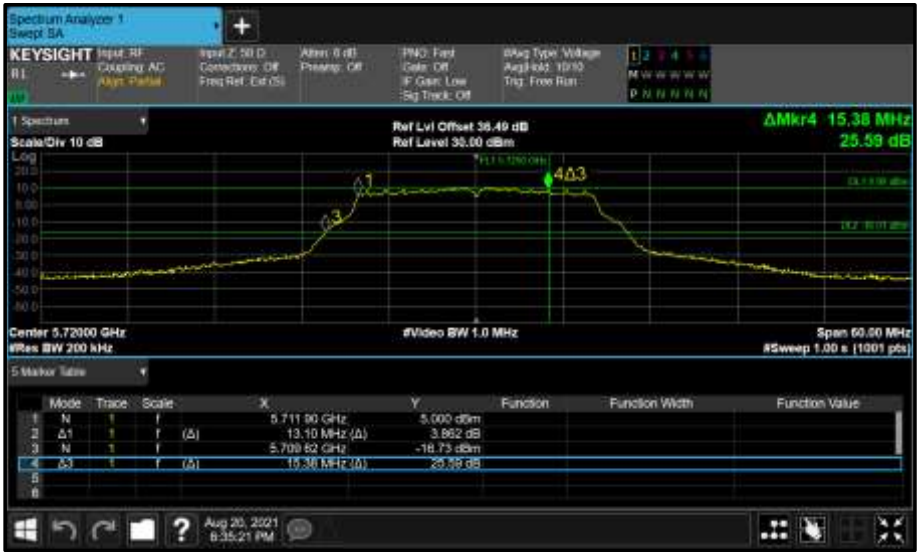
Figure 433 - Core 0 (A) 5720 MHz (CH144) 26 dB and 99% Bandwidth
