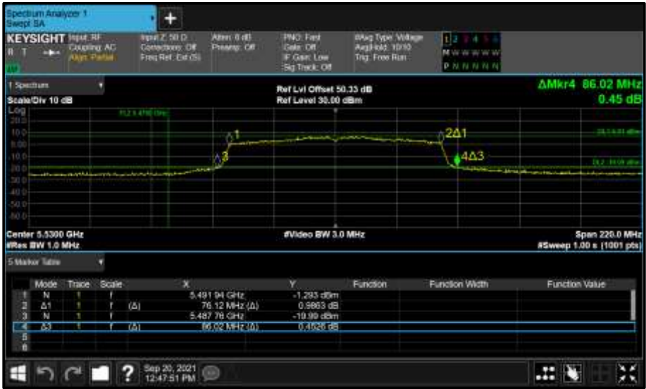
Figure 596 - Core 1 (B) 5530 MHz (CH106) 26 dB and 99% Bandwidth
