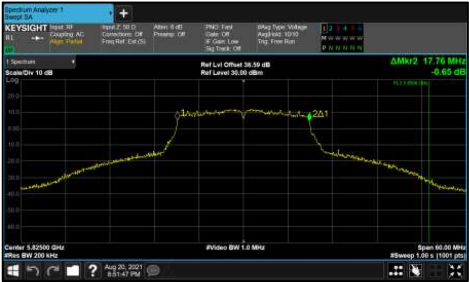
Figure 631 - Core 1 (B) 5825 MHz (CH165) 99% Bandwidth
