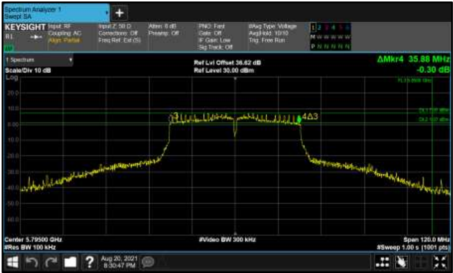
Figure 654 - Core 1 (B) 5795 MHz (CH159) 6 dB Bandwidth
