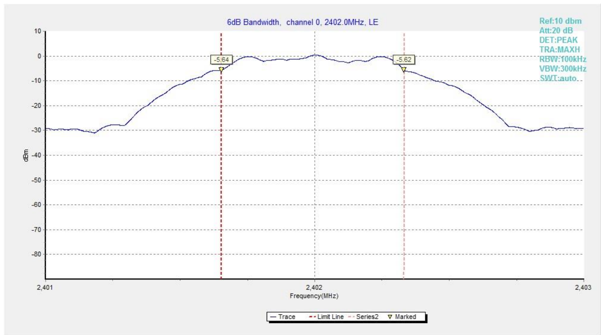
Fig.4 6dB Bandwidth (Ch 0), 1M
