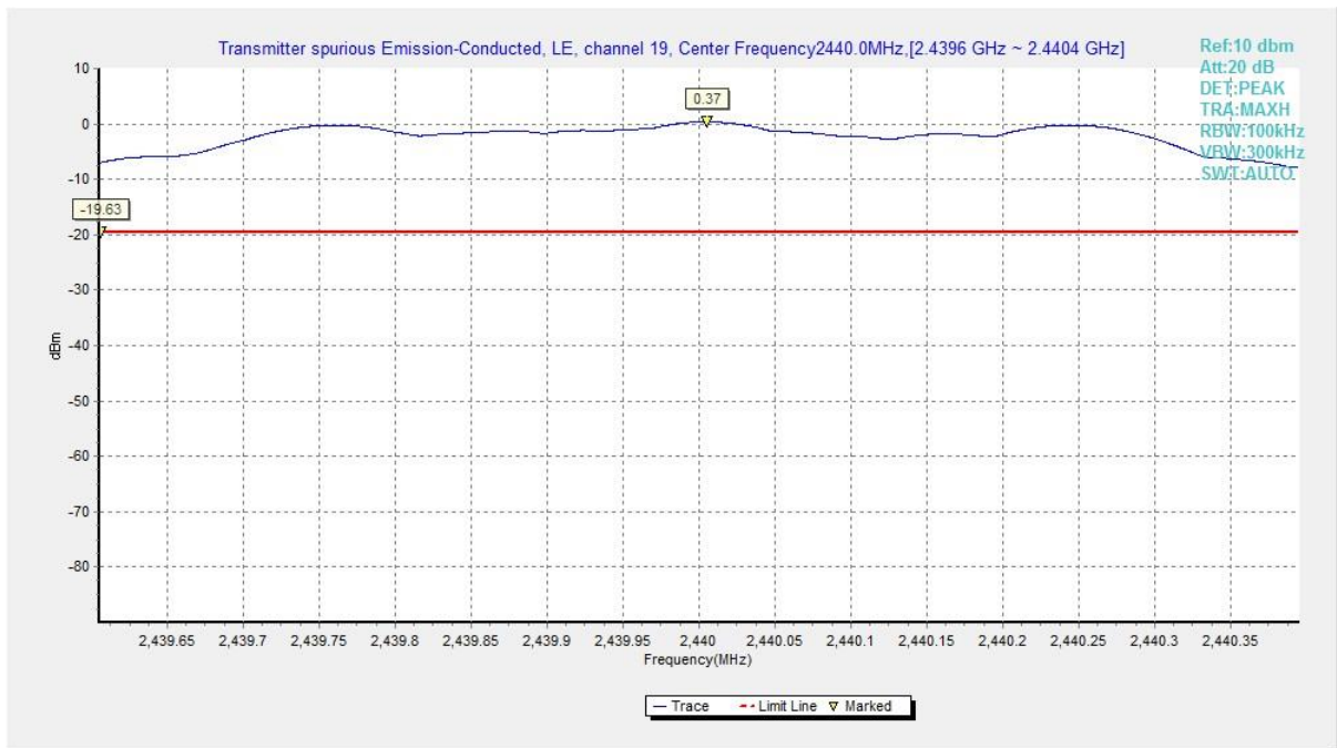
Fig.12 Conducted Spurious Emission (Ch19, Center Frequency), 1M
