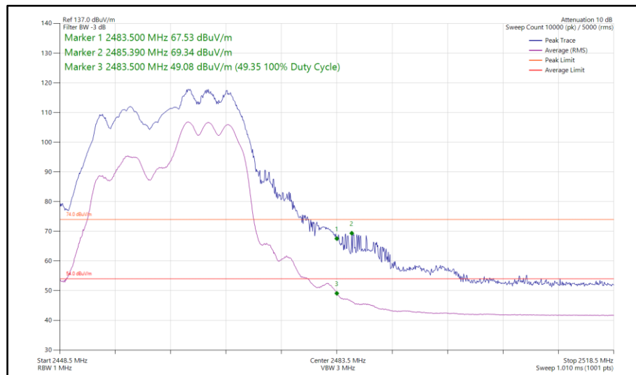
Figure 48 - 802.11ax, HE20, RU 106-54, CDD, Core 0-1 - 2462 MHz, Band Edge Frequency 2483.5 MHz
