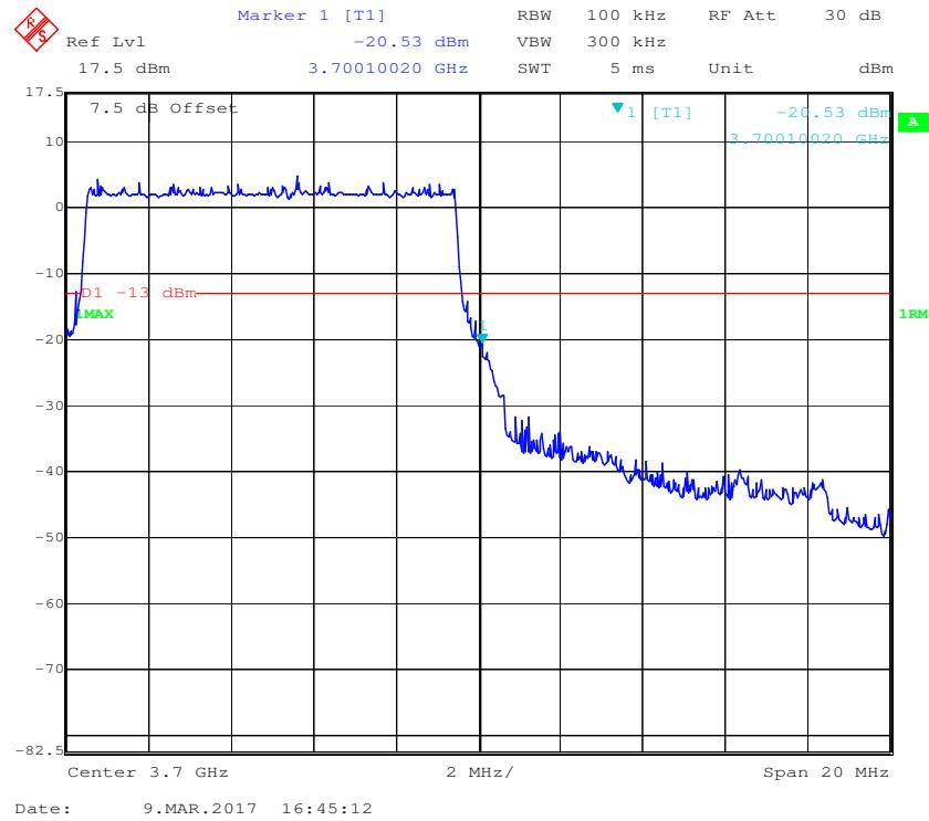
**16QAM (10MHz), Left Side**
