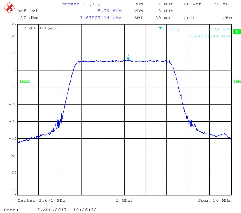
**QPSK (15MHz), High Channel**
