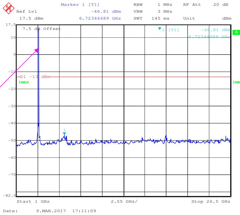
**16QAM(5M)(Channel 1 GHz-26.5 GHz)**
