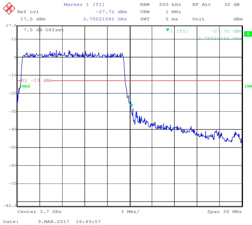
**QPSK (20MHz), Left Side**
