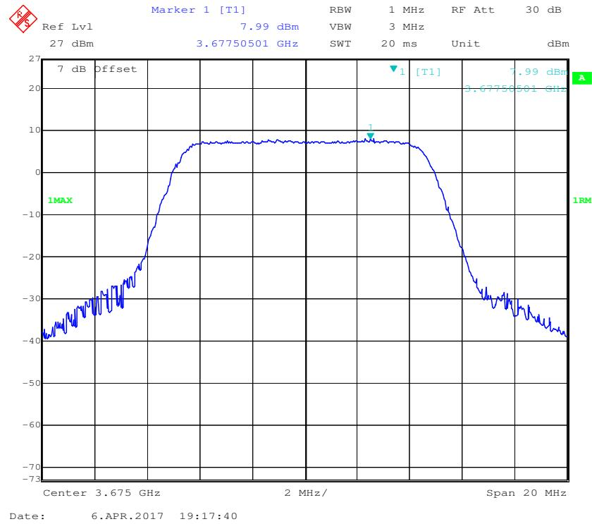
**QPSK (10MHz), High Channel**
