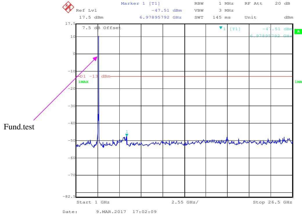
**16QAM(20M)(Channel 1 GHz-26.5 GHz)**
