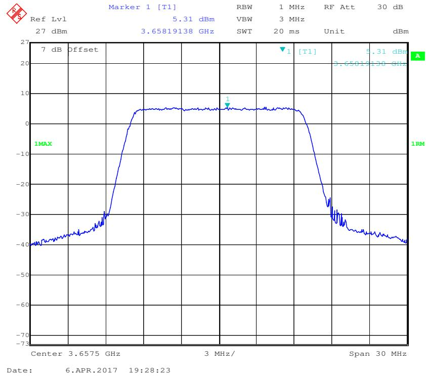
**16QAM (15MHz), Middle Channel**
