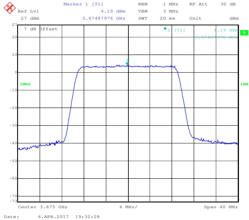
**QPSK (20MHz), High Channel**
