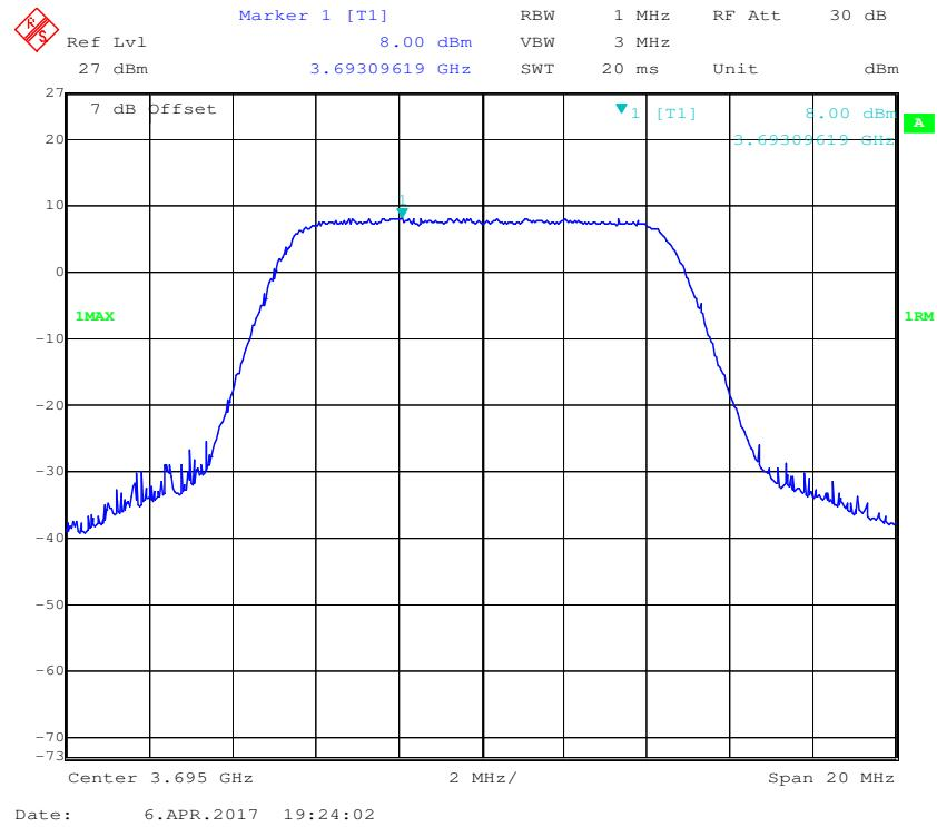
**QPSK (15MHz), Low Channel**
