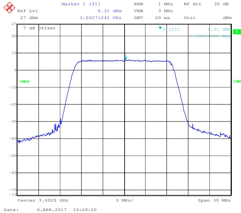
**QPSK (20MHz), Low Channel**
