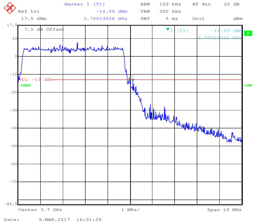
**QPSK (10MHz), Left Side**
