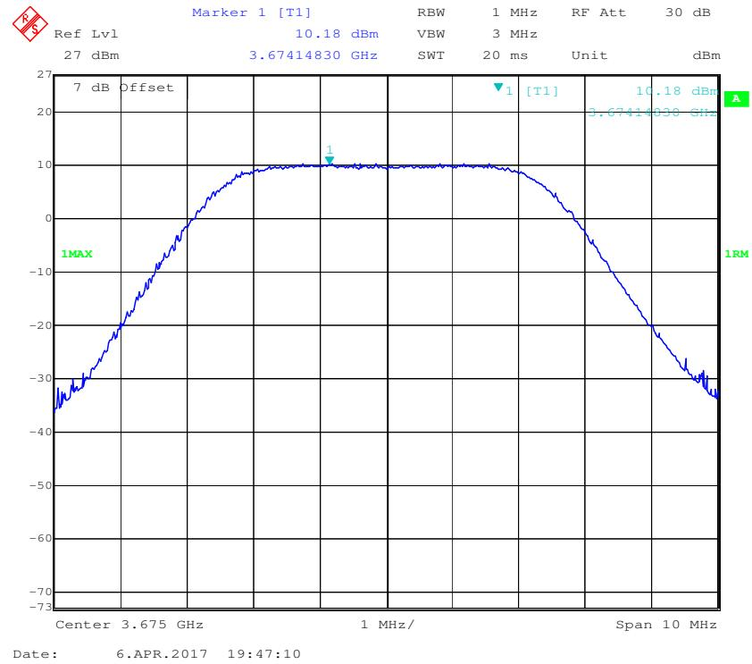
**QPSK (5MHz), High Channel**
