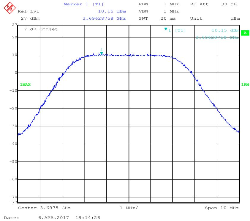
**QPSK (10MHz), Low Channel**
