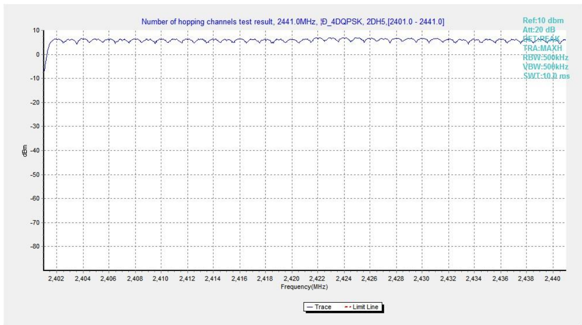
Fig.96. Number of hopping frequencies: \pi/4 DQPSK, Channel 0 - 39
