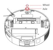
**2** Rinse the wheel and axle to remove hair or dirt. Dry it and reattach the wheel, pressing it firmly into place.
