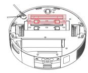
2 Remove the Anti-Tangle Rubber Brush, pull out the bearings at both ends, and clean any hair or dirt wrapped around the brush. You can use the provided small cleaning tool for this.
