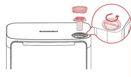
2 Remove the Waste Filter inside, and rinse it under a tap.
