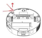
2 Clean the Side Brush and its mounting shaft, then reinstall it.
