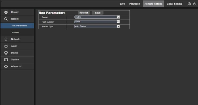
This function is to control the record, pre record and record type (main stream and substream)
