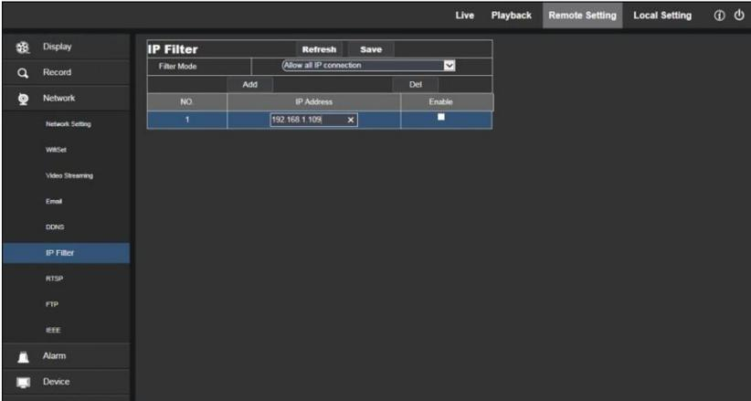
**Filtering mode:** Three modes are available (Allow all IP connections, Allow all IP connections as set, Forbid IP connection as set).
