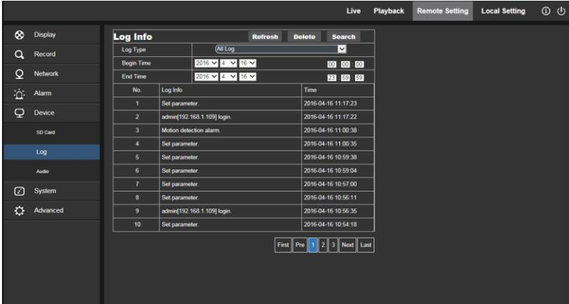
**Log Type:** Eight types of logs are available - system logs, network logs, parameter logs, alarm logs, user logs, recording logs, storage logs and all logs). Choose the starting and ending date/time for retrieval.
