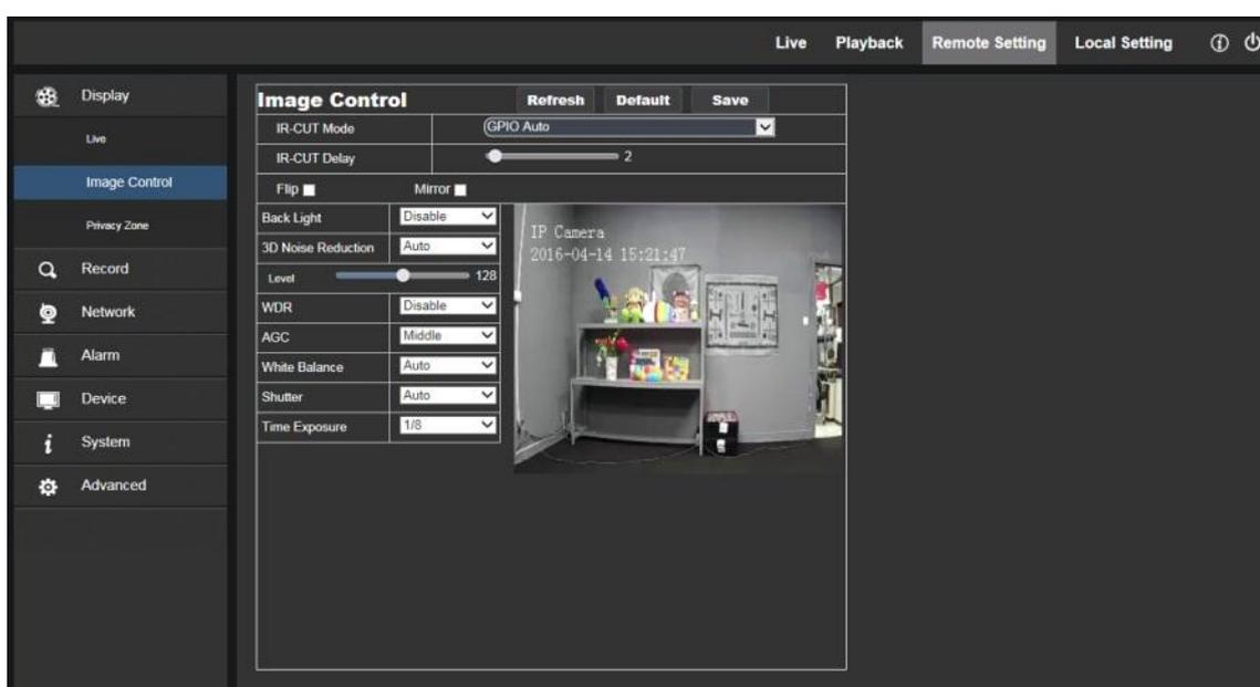
**IR-Cut Model:** Classified into GPIO Automatic, Colored, and Black-White models.
