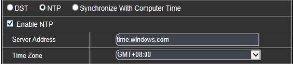
**Sync with PC Time:** The device will use PC as a time server to correct time.
