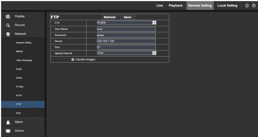
**FTP:** FTP service setting - used with alarm function to upload images or videos snapped to the FTP server.
