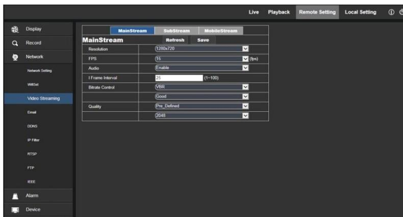
**By default the available bit streams are:** main bit stream, sub-bit stream and cell phone bit steam.
