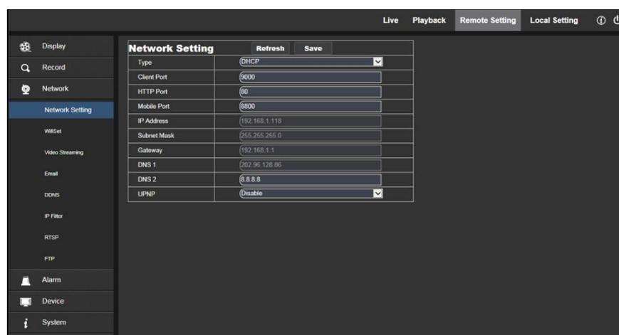
**Networking mode:** DHCP (Automatically Acquired), Manually Configured and PPPOE; the default is DHCP (Automatically Acquired)
