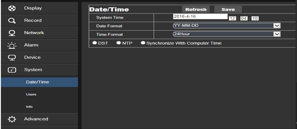
The device time, system time, date format and time format contained in the basic information can be manually set and saved.
