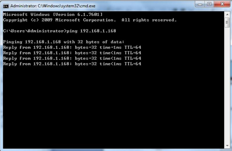
Check whether the IP camera is accessible. If the PING command is executed successfully, it indicates that the IP camera operates normally and the network is connected properly. If the PING command fails, check IP address and gateway setting of the PC and connectivity of the network.
