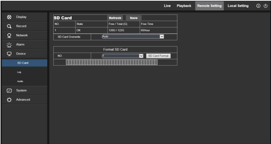
Insert SD card to device, system will auto detect the total capacity and balance capacity of SD card and give The information of time to record
