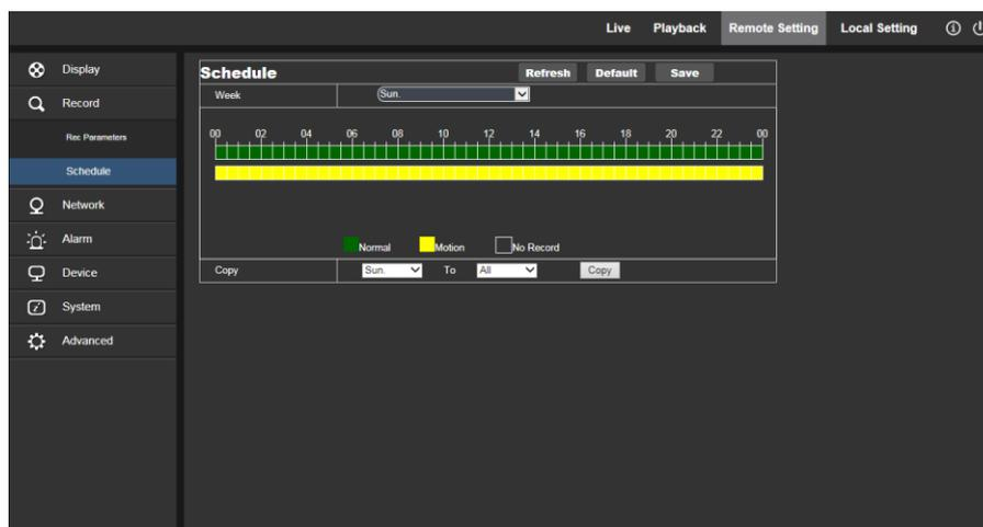
As image: one grid in the table is 30 minutes, green is normal record, yellow is motion detection alarm. User can setup according to private requirement to choose different record type and time.
