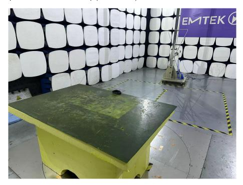
Spurious Emission Test Setup (Above 1GHz)
