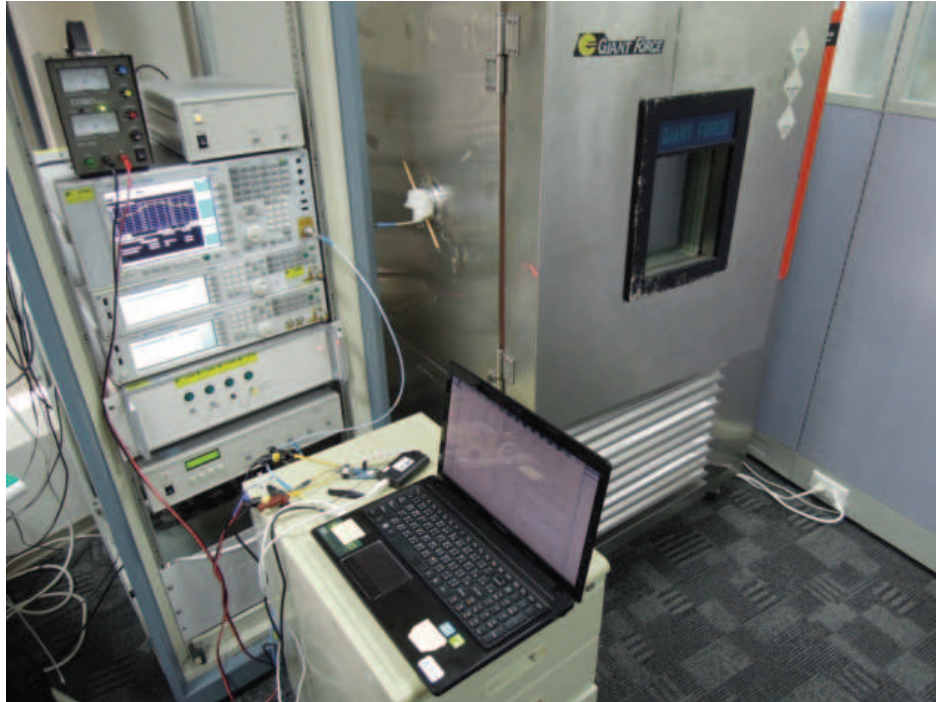
Photograph 27: Set-up for Mains Conducted testing (Front View)
