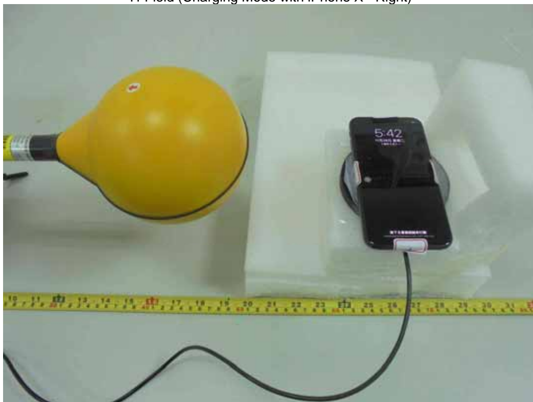
H-Field (Charging Mode with iPhone X - Right)
