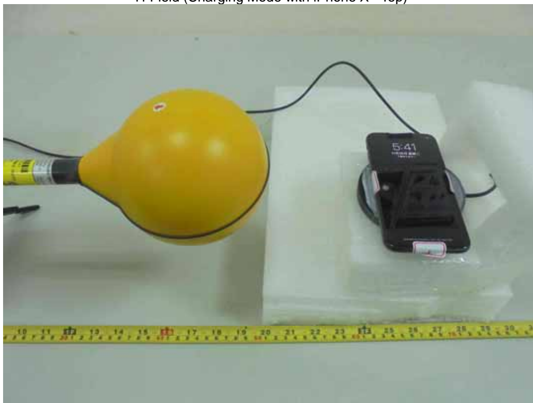
H-Field (Charging Mode with iPhone X - Bottom)
