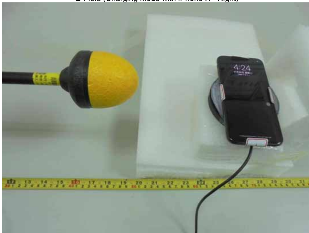
E-Field (Charging Mode with iPhone X - Top)
