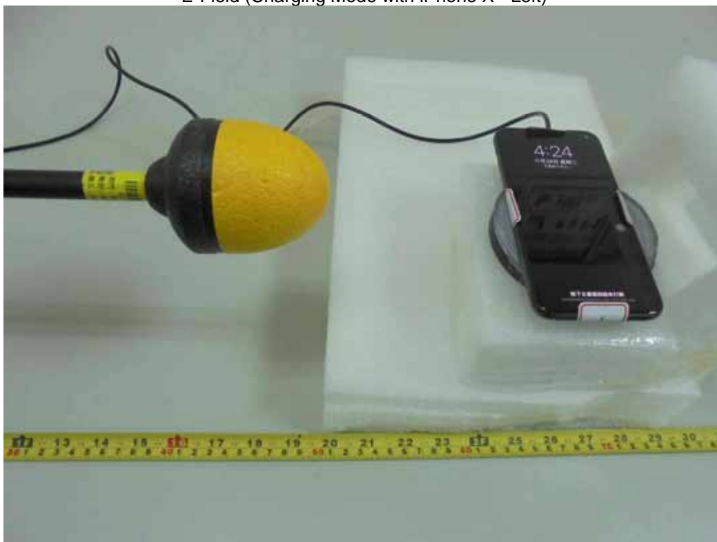
E-Field (Charging Mode with iPhone X - Left)
