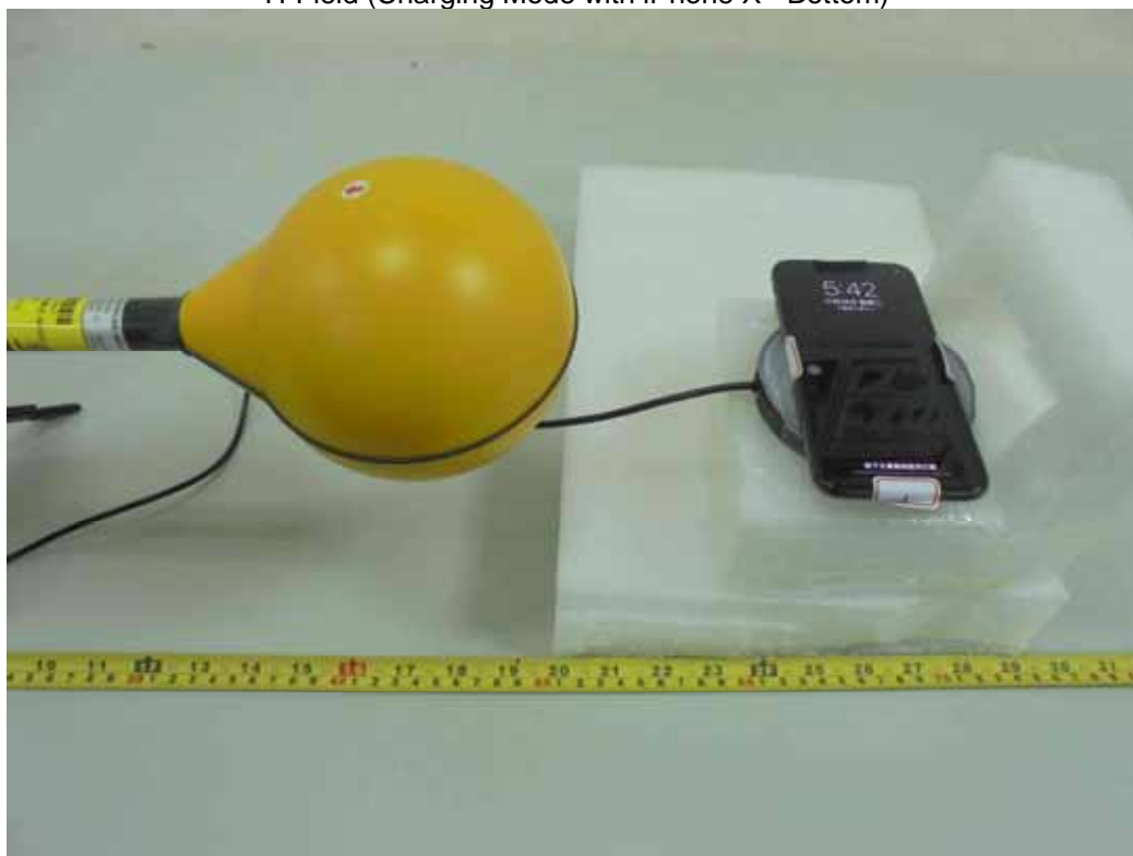
H-Field (Charging Mode with iPhone X - Bottom)
