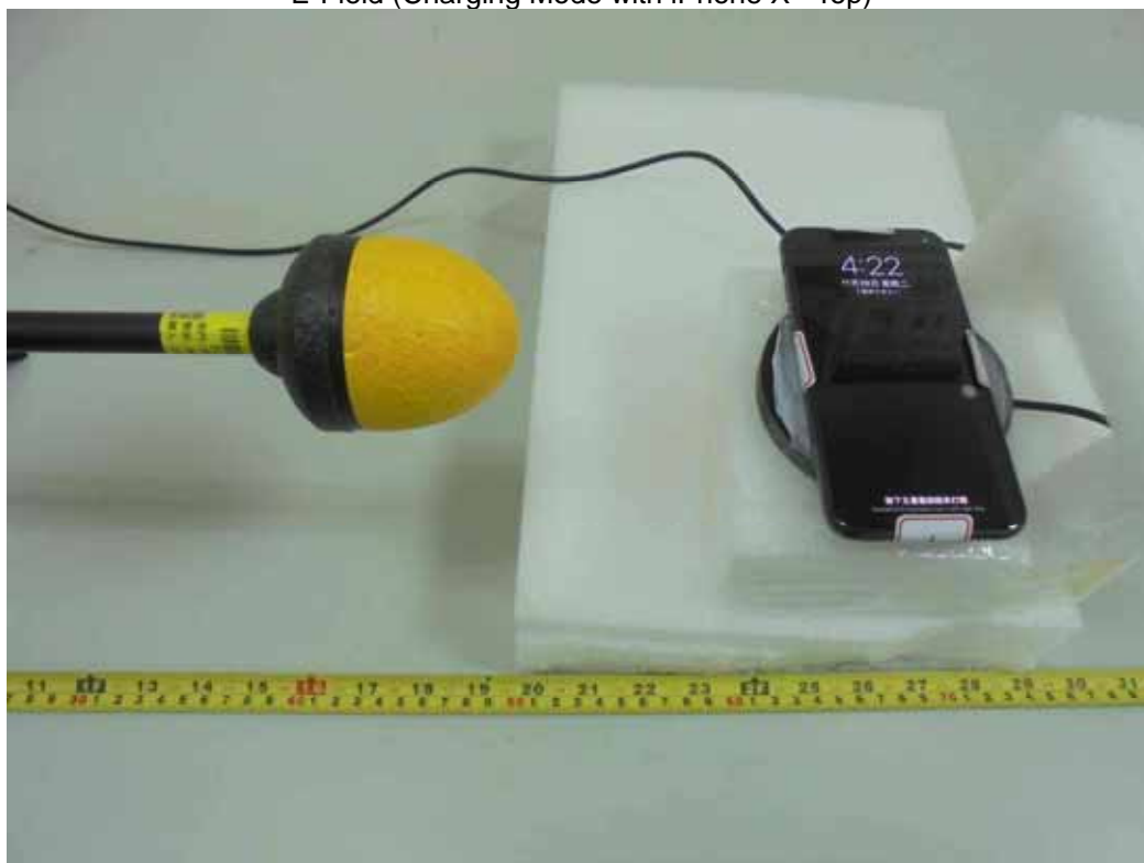
E-Field (Charging Mode with iPhone X - Top)
