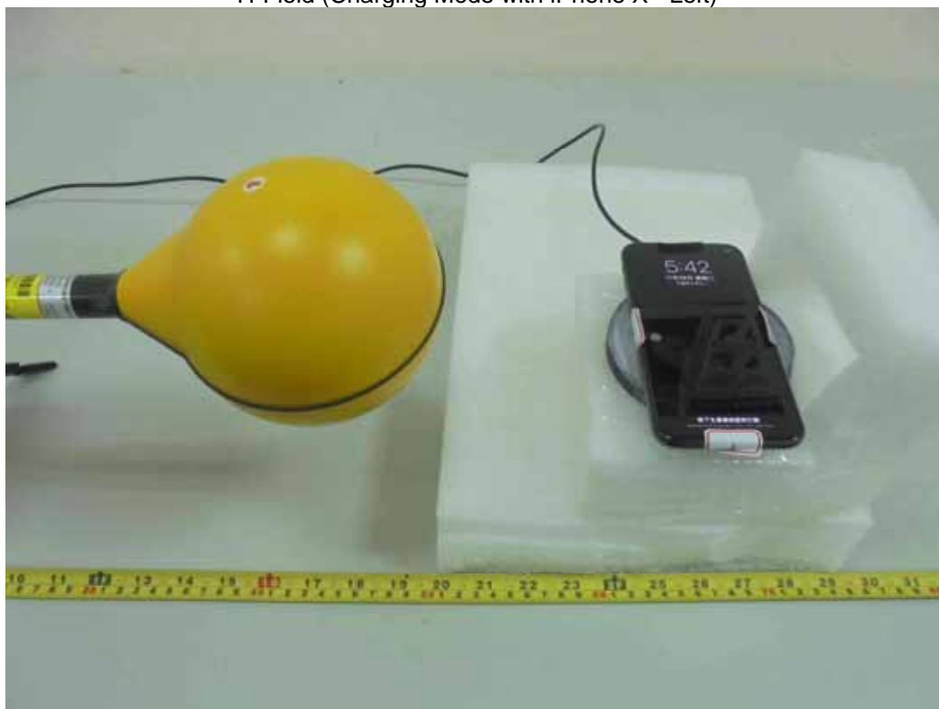
H-Field (Charging Mode with iPhone X - Right)
