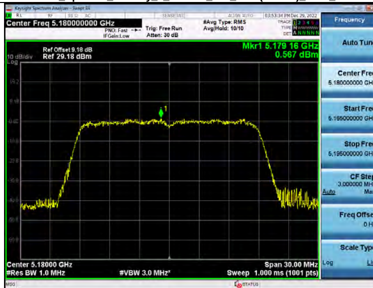
Power Spectral Density 5_2GWiFi_802_11ac(VHT20)_5180_20M
