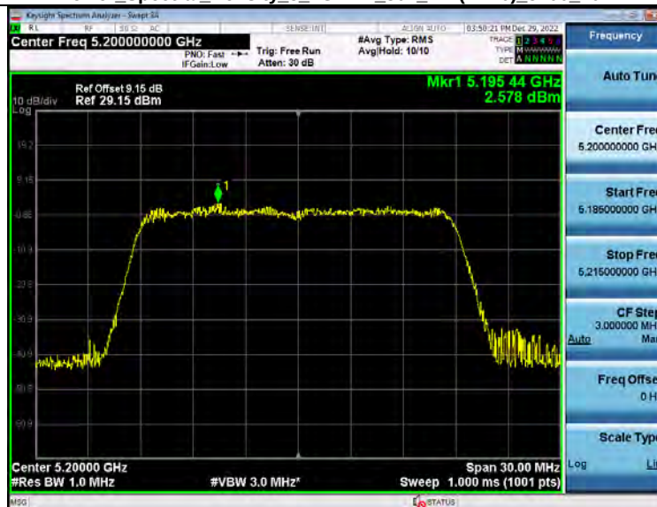
Power Spectral Density 5_2GWiFi 802_11n(HT20) 5200_20M
