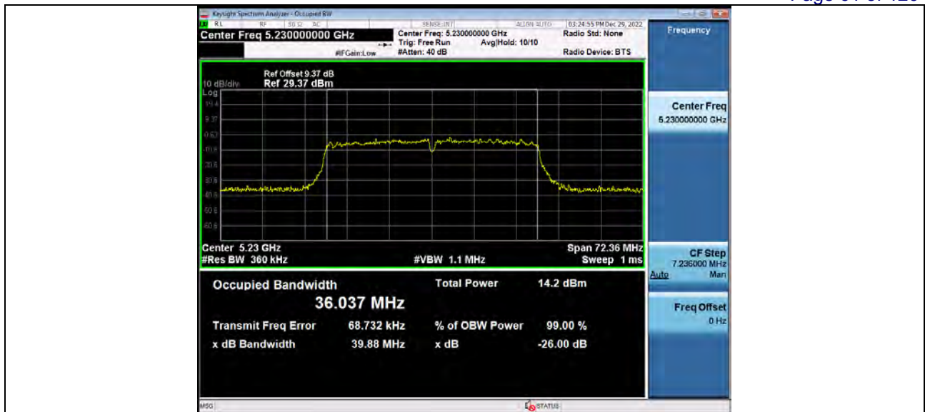
-26dB and 99% Emission Bandwidth 5 2GWiFi NVNT ANT1 802_11ac(VHT40) 5190_40M
