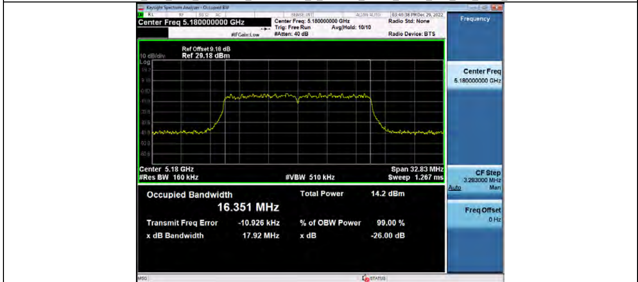
-26dB and 99% Emission Bandwidth 5 2GWiFi_NVNT_ANT2_802_11a_5180_20M
