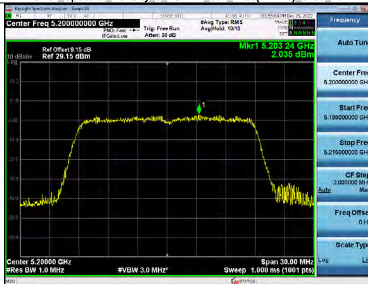
Power Spectral Density 5_2GWiFi_802_11ac(VHT20)_5200_20M
