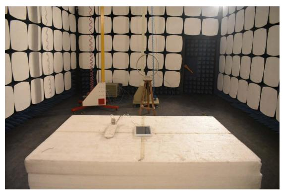
3. Radiated emission (9KHz-30MHz)
