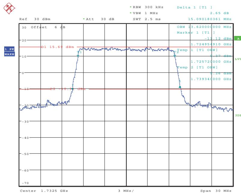
**16-QAM (15.0 MHz) - 26 dB Bandwidth & 99% Occupied Bandwidth, Middle channel**
