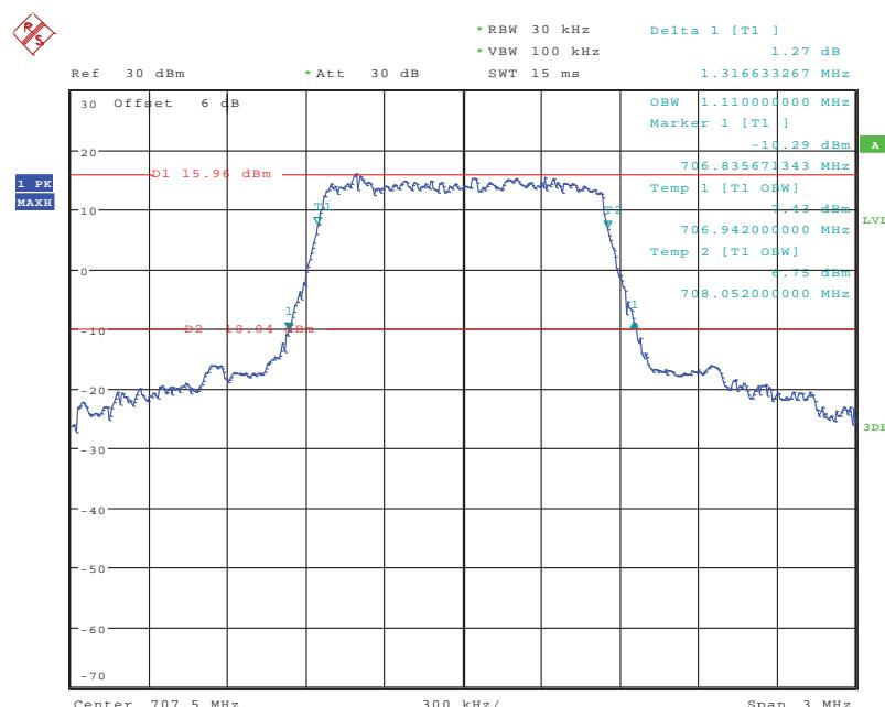
**QPSK (3.0 MHz) - 26 dB Bandwidth & 99% Occupied Bandwidth, Middle channel**
