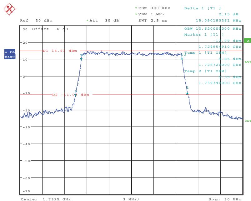
**QPSK (20.0 MHz) - 26 dB Bandwidth & 99% Occupied Bandwidth, Middle channel**
