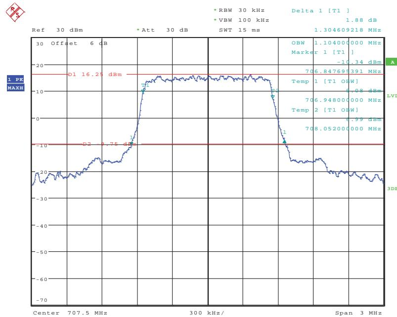
**16-QAM (1.4 MHz) - 26 dB Bandwidth & 99% Occupied Bandwidth, Middle channel**
