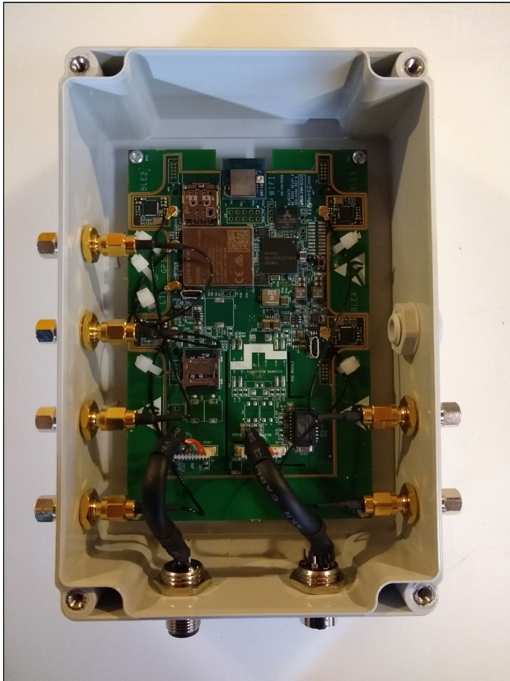
Photograph 1. EUT – Front Cover Removed
