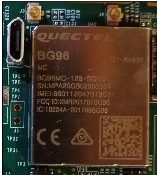
Photograph 4. Cellular Module (Quectel BG96)
