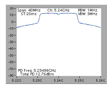
Power Density Plot on Configuration IEEE 802.11n MCS8 HT40 / Chain 1 + Chain 2 / 5230 MHz
