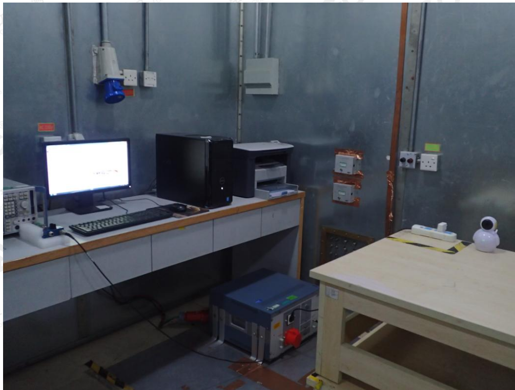
RADIATED EMISSION TEST SETUP BELOW 1GHZ
