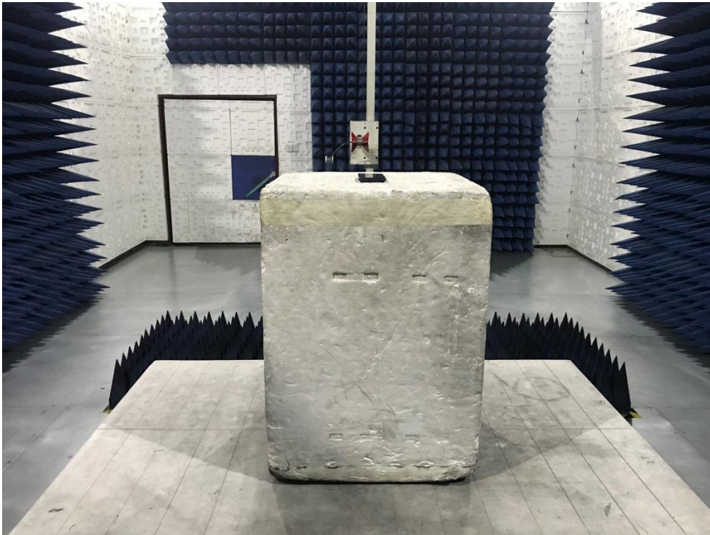
RADIATED EMISSION TEST SETUP ABOVE 1GHz
