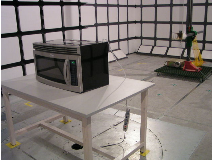
Above 1 GHz-Radiated Emission–Front View
