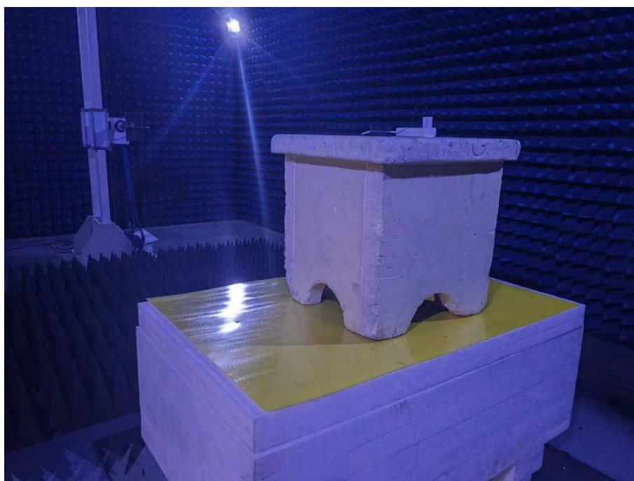
Photo of Radiated Emission Measurement Above 1GHz
