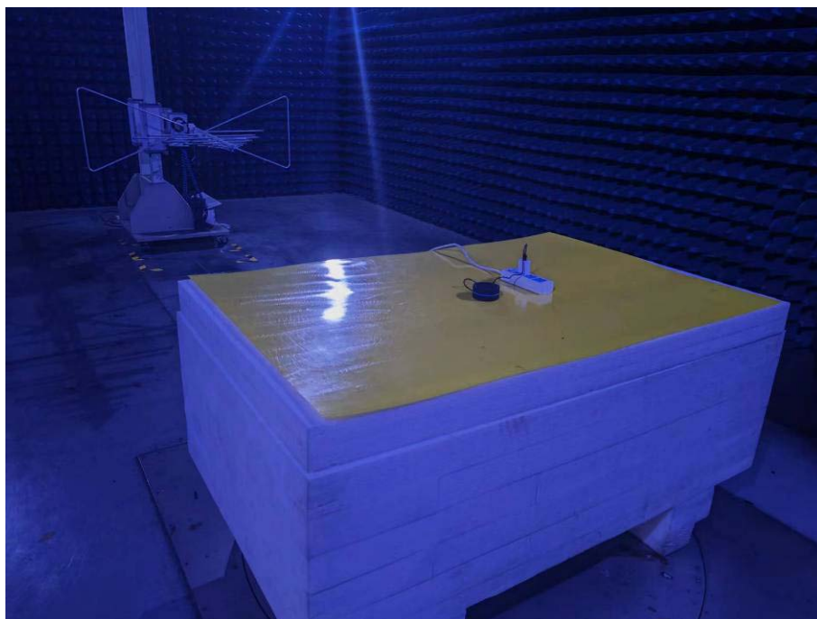
Photo of Radiated Emission Measurement Below 1GHz
