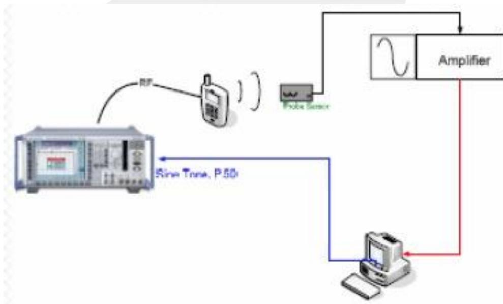
T-Coil Test Setup
