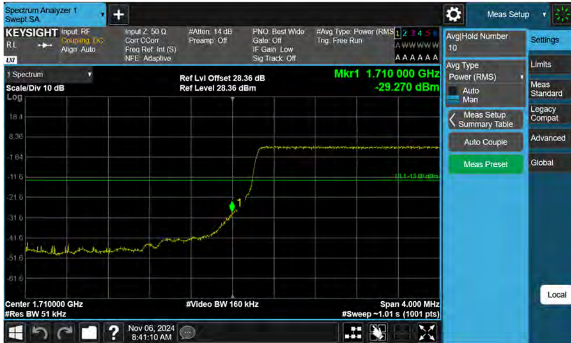
NR66_5 M_Band Edge_Low_BPSK_FullRB
